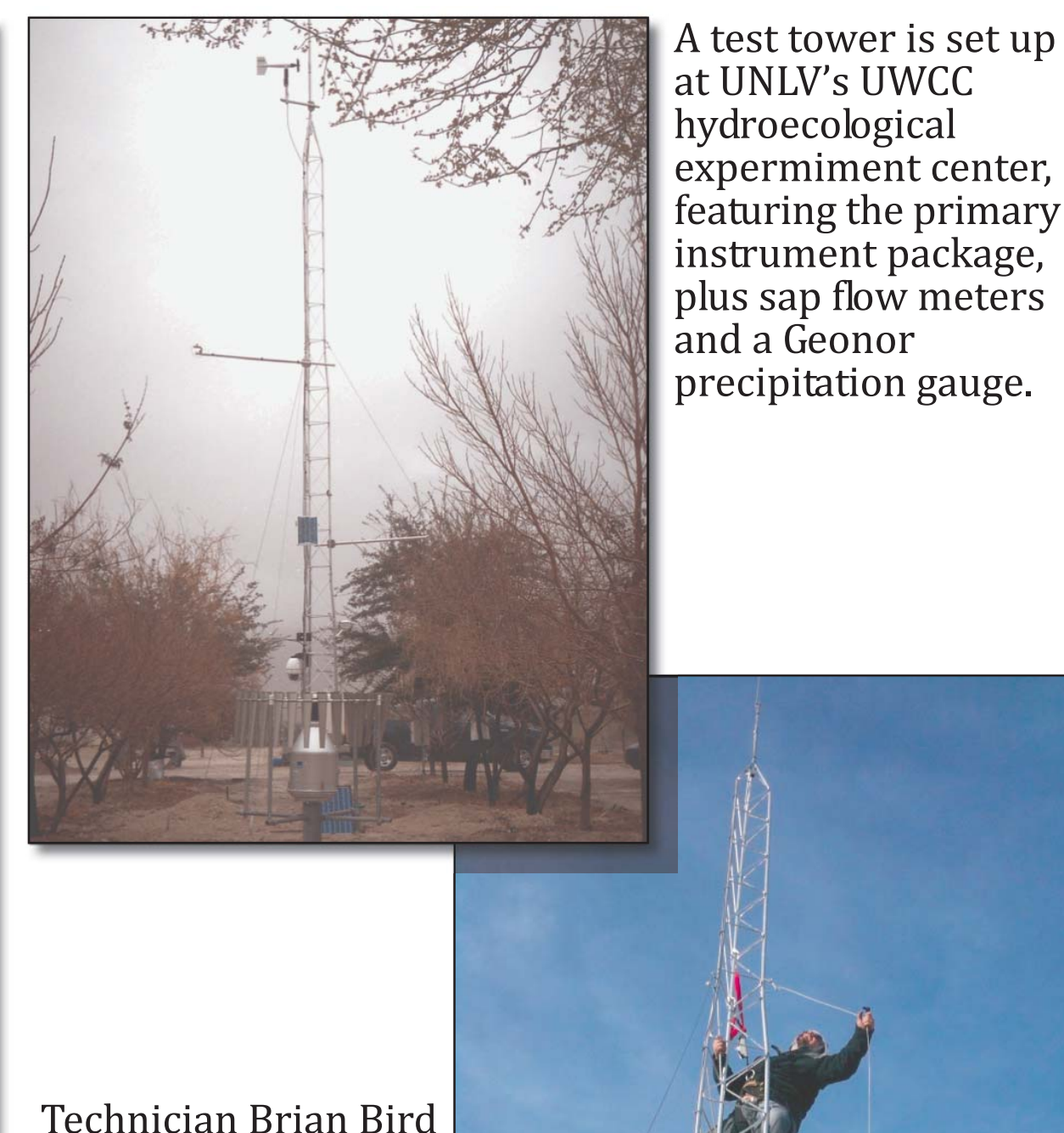
Technician Brian Bird configuring the UNLV test tower. Instrument towers at most of the sites will be 10m in height, and support the meteorological sensors in addition to solar arrays and communications antennas.
