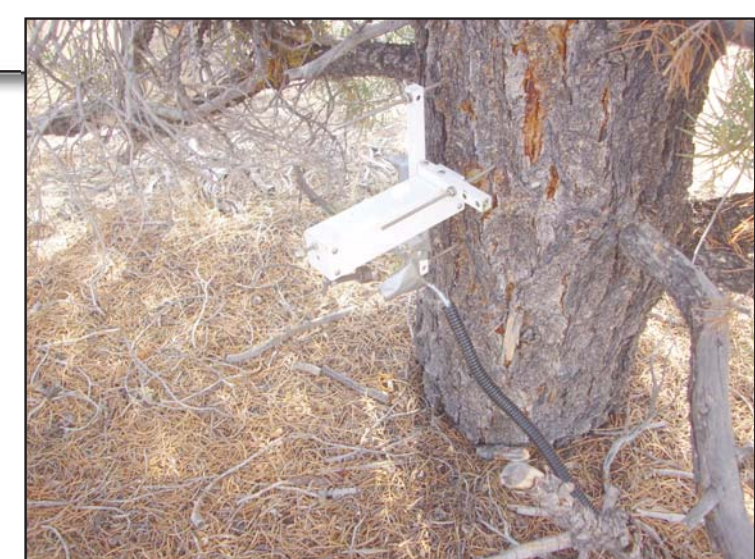
This point dendrometer is recording incremental radial tree growth at 30min intervals as part of a site located in Pinyon-Juniper woodland in Great Basin National Park.
