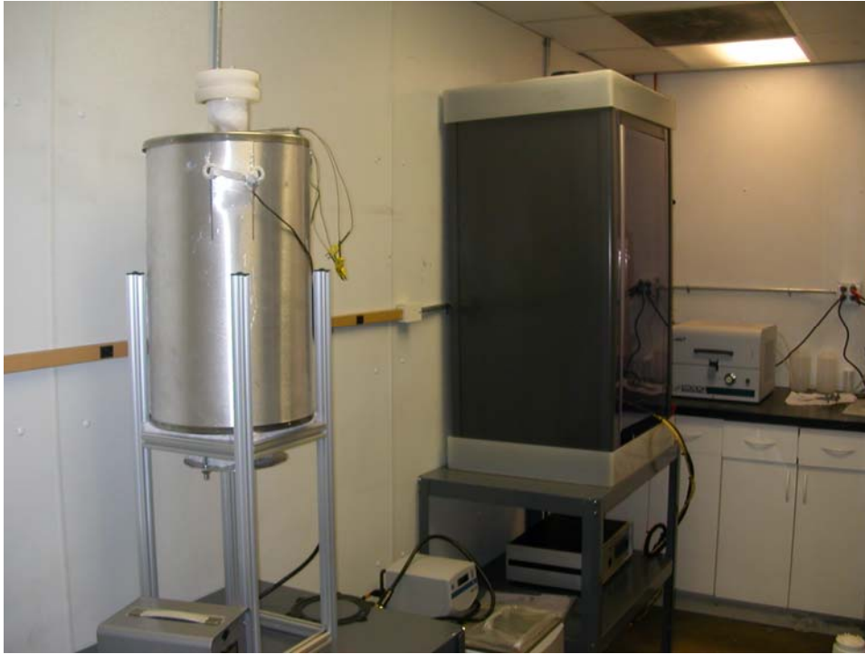
Figure 1. High Temperature Corrosion Exposure Test Rigs at Ceramatec, Inc.
