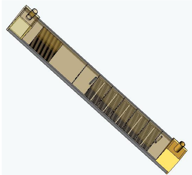
Figure 15. Schematic Diagram of a Single-Chamber Test Section for the Off-set Strip Fin Plate Type Heat Exchanger.
