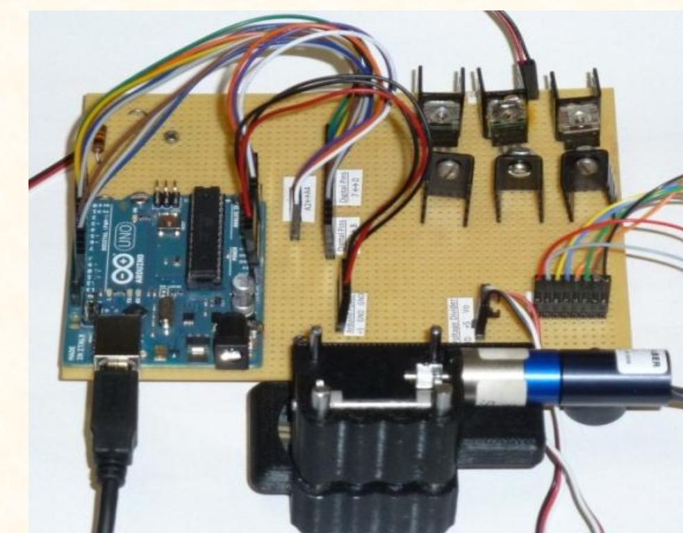
Arduino Board is used to control the Commutation
