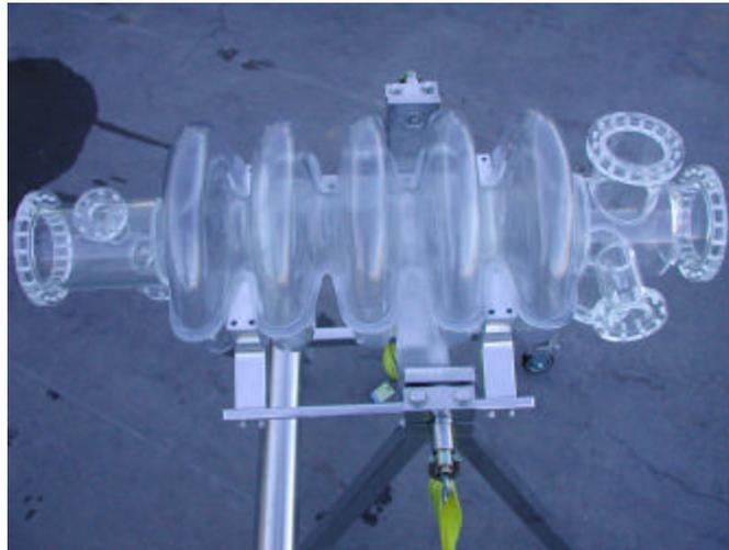
**Figure 7.** Photo of the LANL Transparent Cavity
