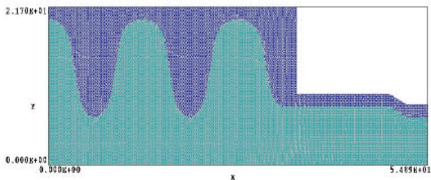
(c) Five-cell niobium cavity original beta 64 LANL cavity geometry
