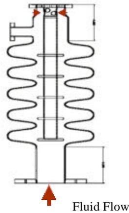
**Figure 4.** Current Etching Configuration of Niobium Cavities
