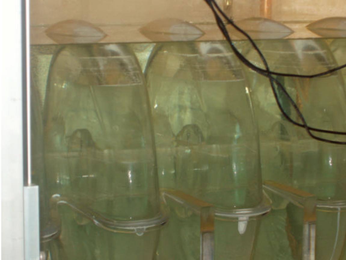
Figure (4.20) Fabricated LANL baffle inside the cavity
