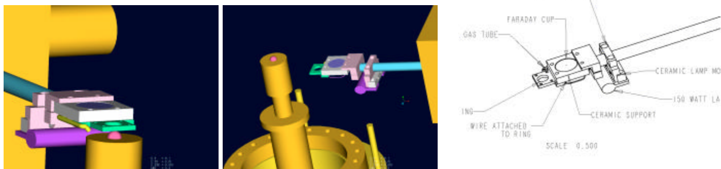
Figure 6. Solid model and a line drawing with labels of the XYZ high vacuum manipulator. The manipulator is being used for a number of purposes: target positioning, primary electron beam charge measurements, primary electron beam positioning, in situ cleaning of carbon based molecules, and in situ cleaning of water molecules.
