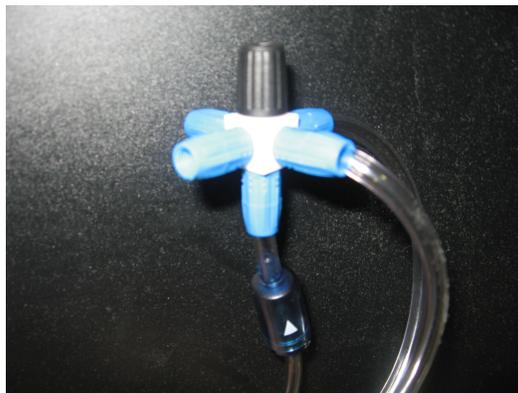
Figure 2.4 Control valve with charcoal filter that filters the incoming air from the oxygen tank. The two oxygen tubes leaving the through the side of the valve, channel the air flow to the scent boxes.
