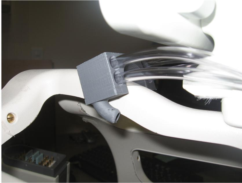
Figure 2.8 Coil mounted delivery device. Oxygen tubes come through the bore of the magnet, entering the device through the caudal end. Oxygen is passed through the tubes and released through the inferior holes, forcing the air in the direction of the nostrils.
