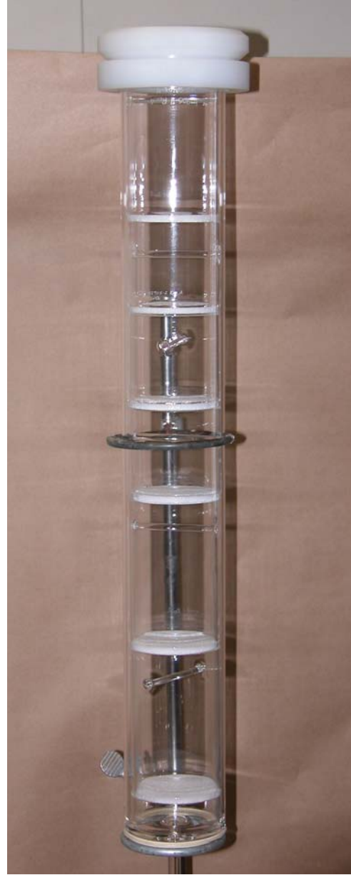
c) Quartz Liner w/ Evaporator, Condenser and Specimen Cups.
