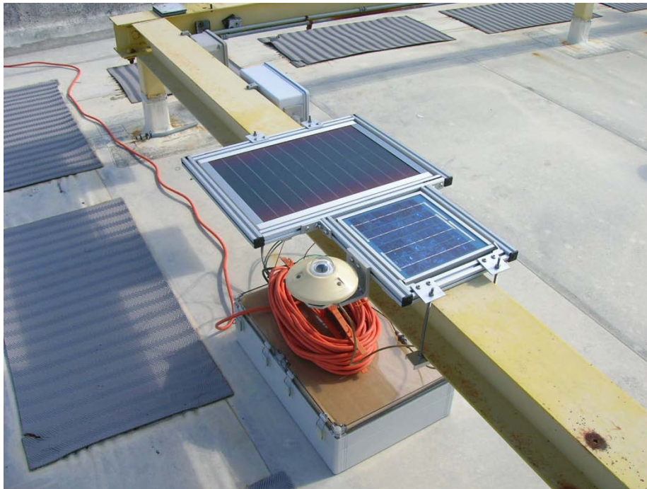
Figure 3-3. BP Solar model SX5M and UNI-SOLAR model US-11 PV modules with plane-of-array pyranometer at FSEC for June 14-19, 2008. PV modules are mounted horizontal and viewed from the north.
