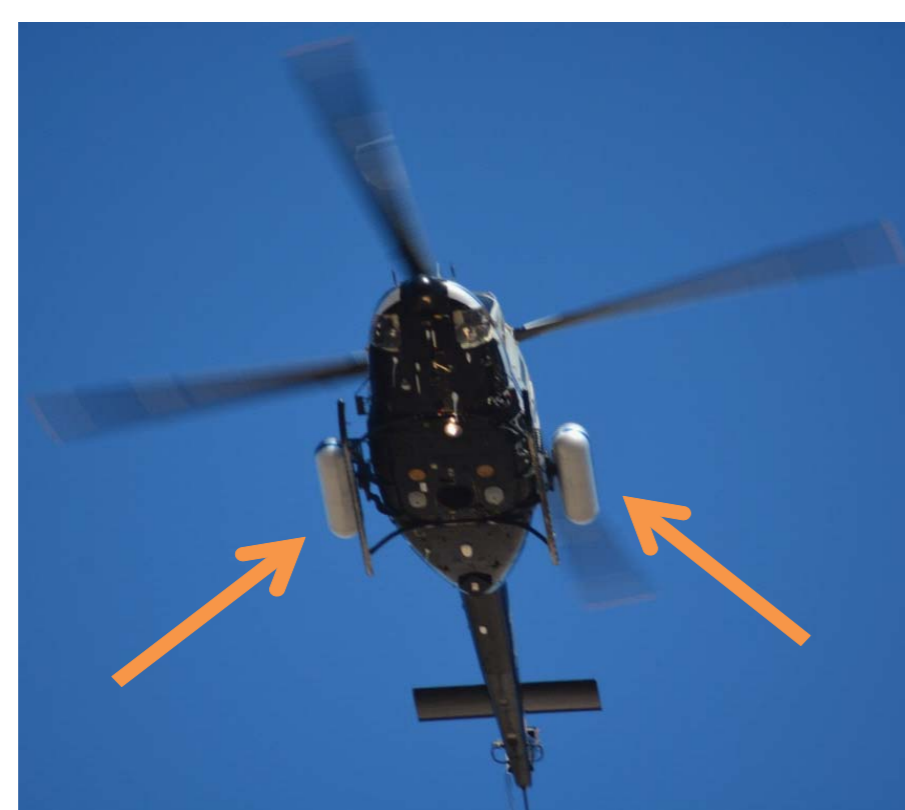
Figure 2: NSTec Helicopter with gamma ray detectors attached
