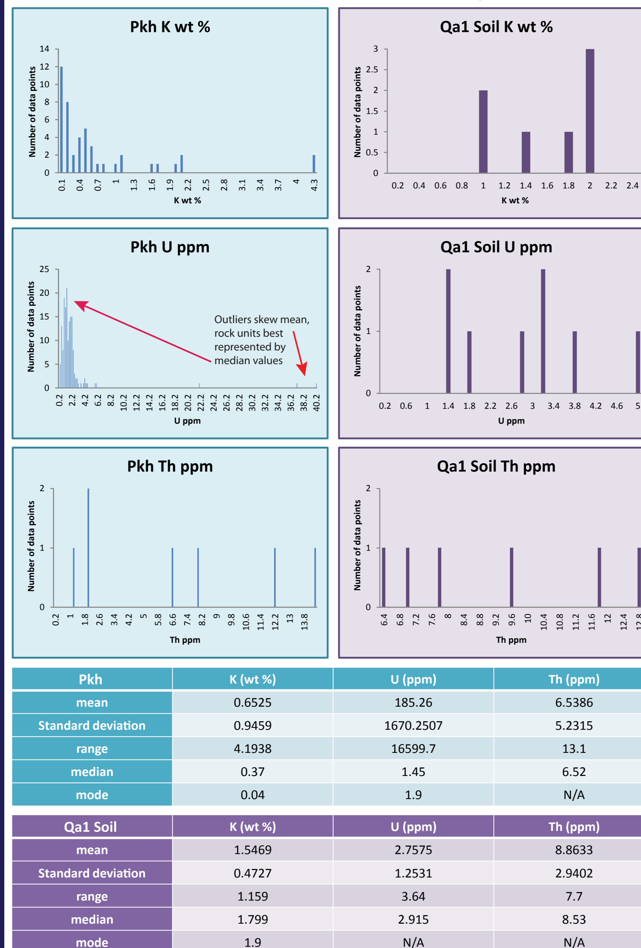
Figure 5: Example rock (blue) and soil (purple) unit reports for Pkh (limestone, Harrisburg Member, Kaibab Fm) and Qa1 (Holocene alluvial fan deposits), includes histograms and statistics of U, K, Th concentration. This is how values were assigned to geologic units with multiple data points.
