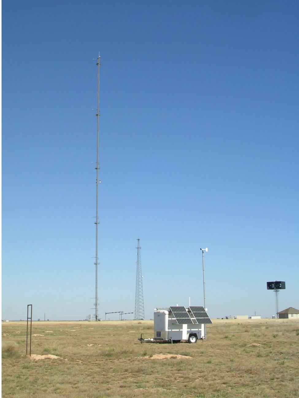
Figure 1. The SODAR and Tower field configuration.
