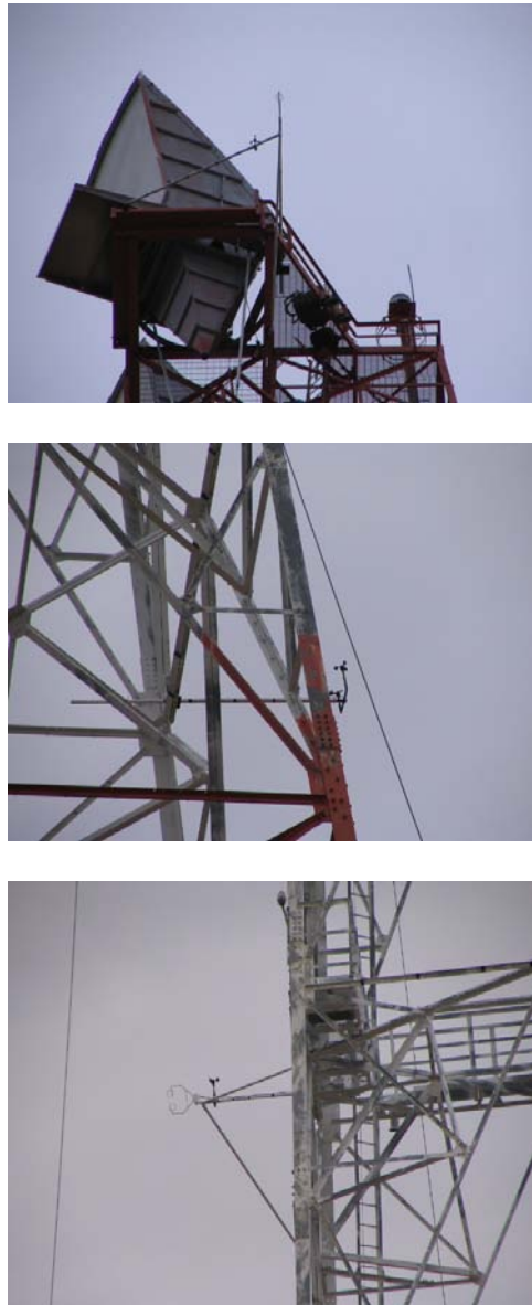
Figure 10. Photos of the mounted standard and sonic anemometers at 40, 60, and 80 m on the Stone Cabin tower
