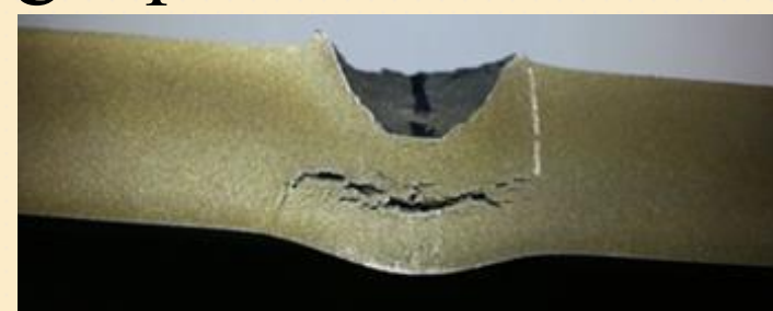
Spalling of target plate (sectioned)
