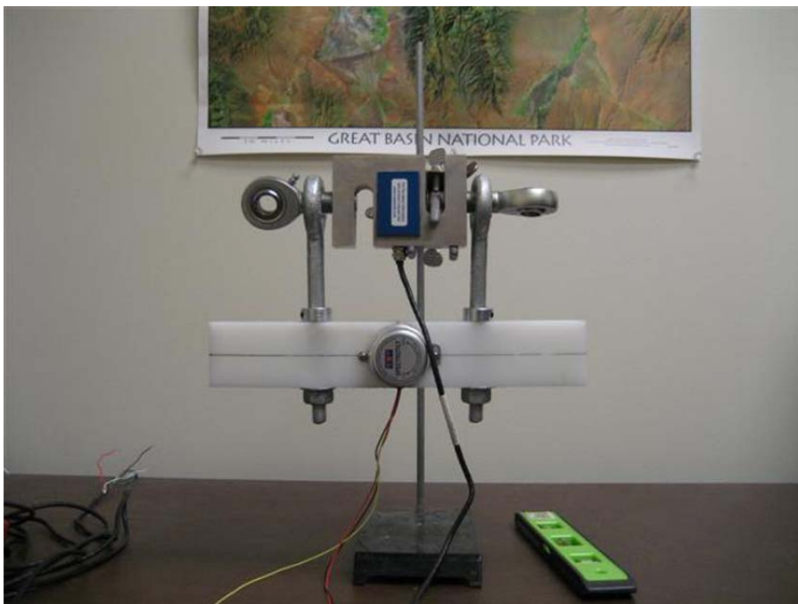
Figure VI. 3. Strain gauge and horizontal inclinometer. The apparatus was attached to the winch pull line and measured both the force applied to the tree and the angle of the pull line.
