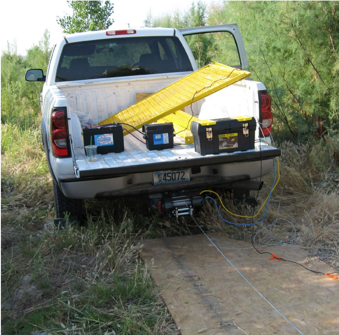
Figure VI.1. Winch used for tree pulling field experiments. The winch was powered by the deep cycle marine batteries located in the truck bed. The black toolbox on the right side of the tailgate houses a CR1000 datalogger. A laptop computer connected to the datalogger enabled real-time monitoring of experimental data.
