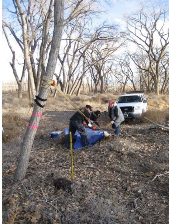
Figure VI. 4. Preparation of the tree pulling apparatus prior to testing conducted on a Rio Grande cottonwood. Note the vertical inclinometer attached to the tree near the winch line attachment on the tree trunk. The strain gauge/horizontal inclinometer apparatus pictured in Figure VI.3 above can be seen hanging from the winch line near the researchers.
