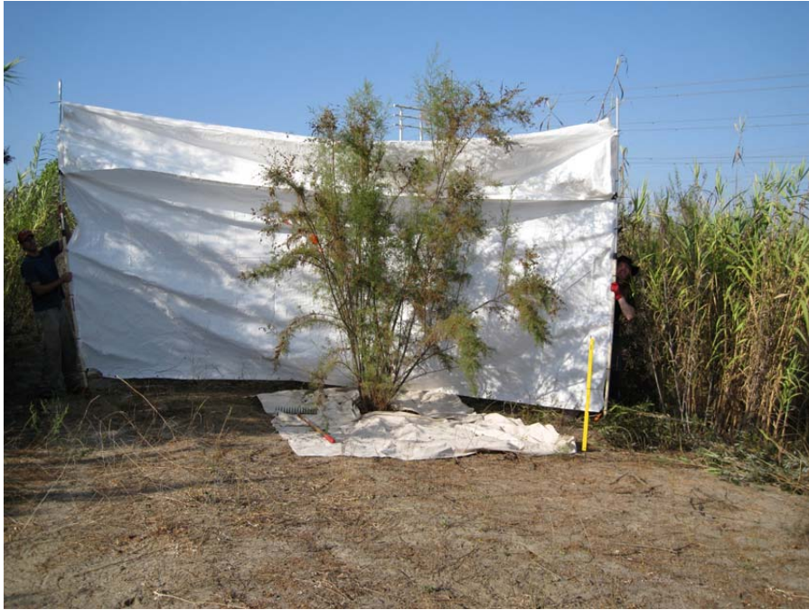
Figure VI. 2. Digital photograph of a San Luis Rey salt cedar used for determination of nonstreamlined frontal area ( A_0 ) and height ( L ). Note the yellow yardstick located to the lower right of the tree for image scaling.
