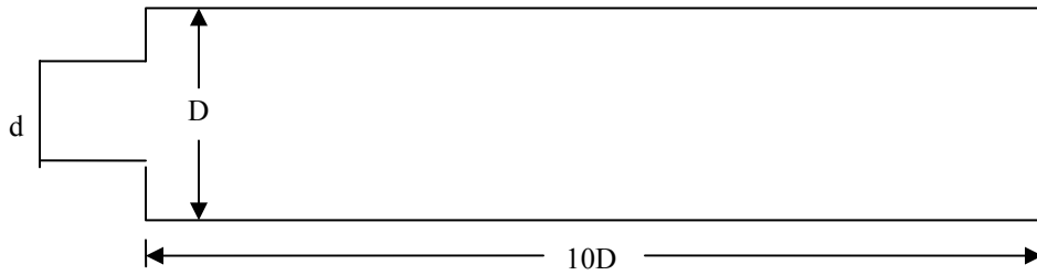
Figure 4. The schematic of sudden expansion pipes
