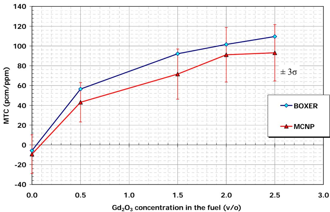
Figure 2. Effect of Gd loading on MTC: Boxer vs. MCNP comparison
