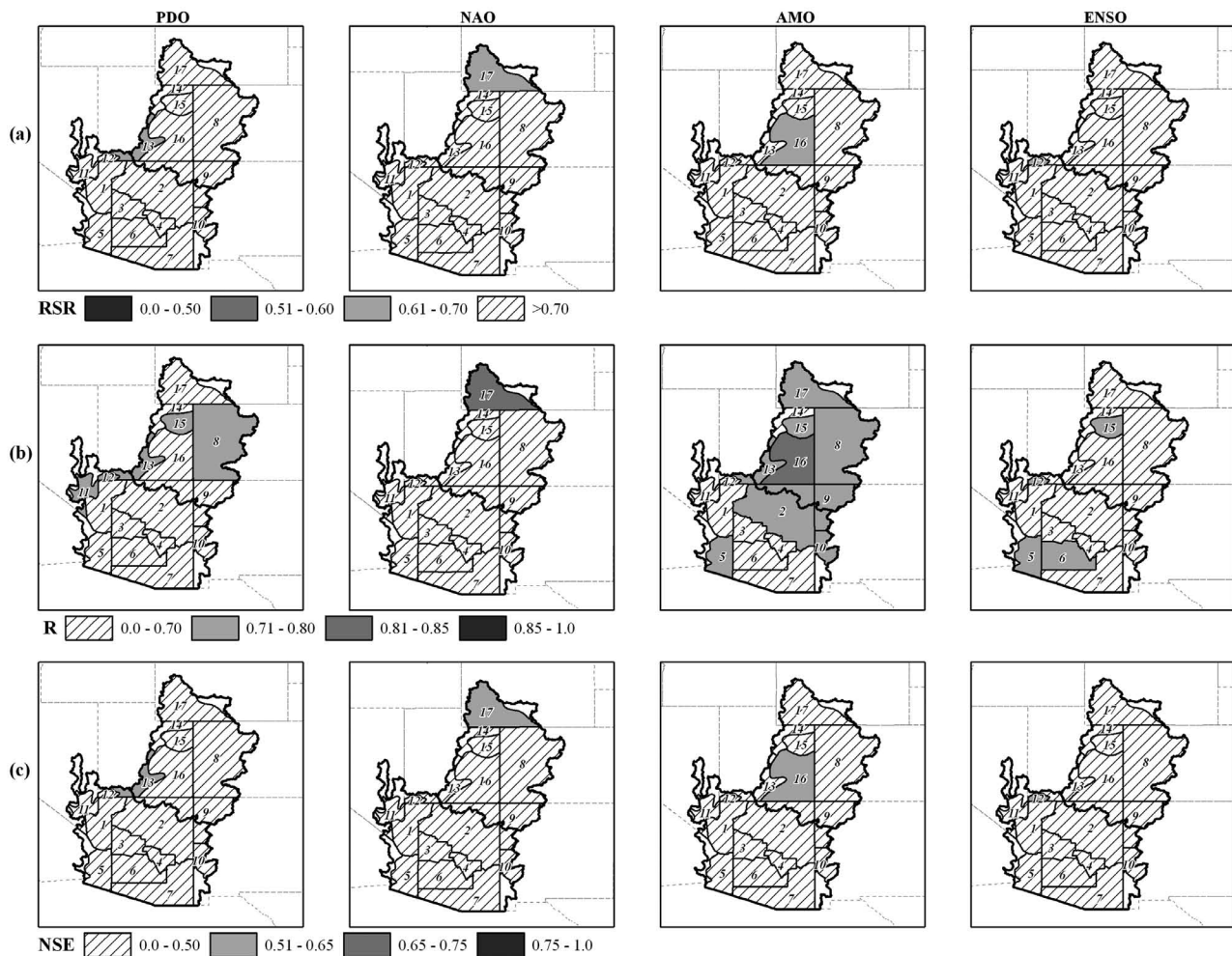
Figure 10. Spatial maps showing the range of performance measures for 17 climate divisions for Model IV: (a) RSR, (b) R, and (c) NSE.
