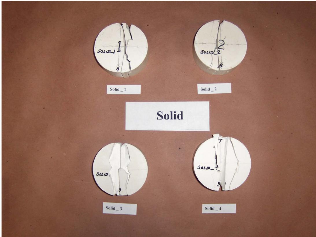
Figure 20 Solid Specimens after Testing
