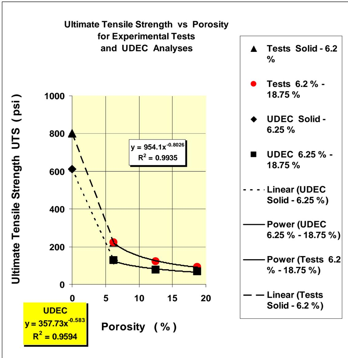
Figure 49 Ultimate Tensile Strengths versus Porosity for TESTS and UDEC
