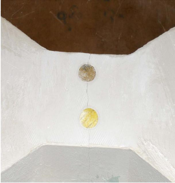
Figure 15 Crack in Dog Bone 4
