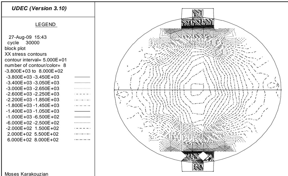
Figure 29 Horizontal Stresses in Solid Model at Failure
