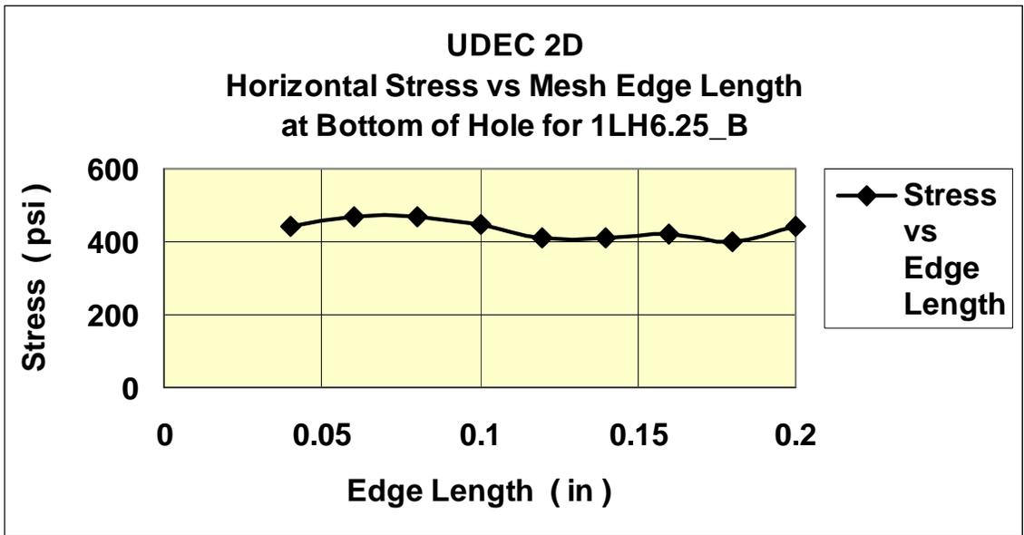
Figure 64 UDEC Horizontal Stress versus Edge Length
