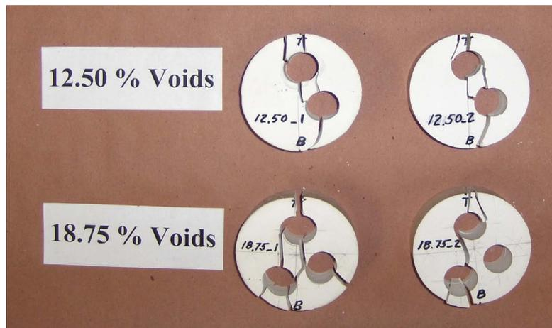
Figure 23 Large Hole 12.50% and 18.75% Voids Specimens after Testing
