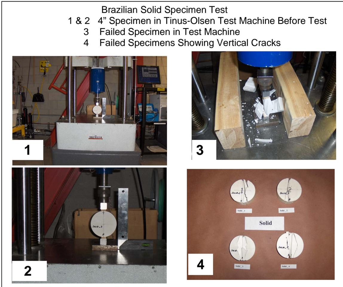
Figure 19 Test in Tinus-Olsen Machine for Solid Specimens
