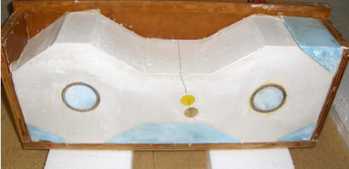
Figure 12 Mold Removal of Dog Bone 3 Showing Crack
