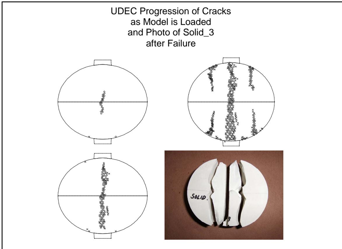
Figure 28 UDEC Solid Models and Test Specimen Solid\_3
