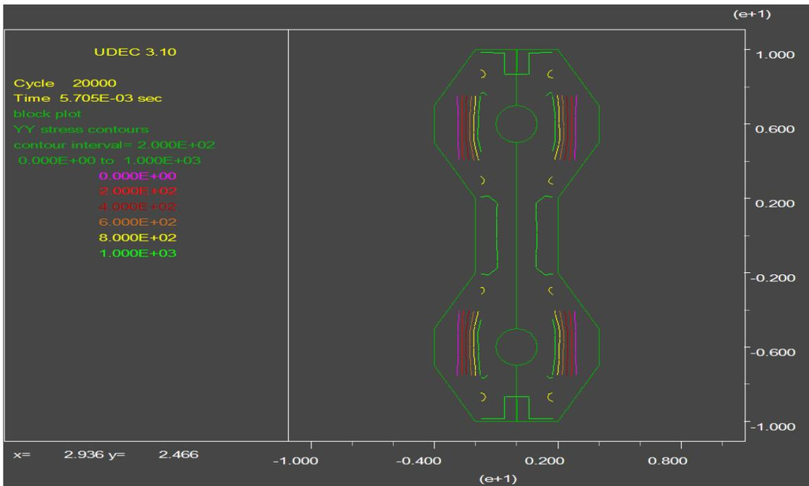
Figure 26 Dog Bone 1 Stresses in the Vertical Direction
