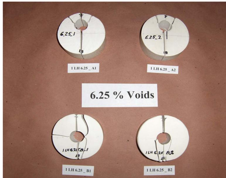
Figure 22 Large Hole 6.25 % Voids Specimens after Testing
