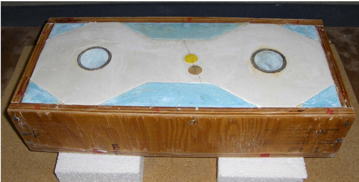
Figure 11 Crack in Dog Bone 3
