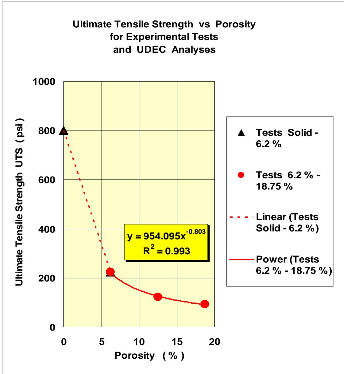
Figure 25 Averages of Ultimate Tensile Strengths versus Porosity
