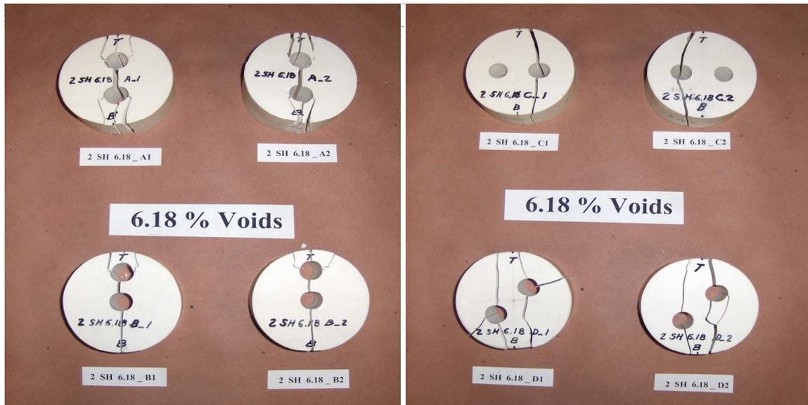
Figure 21 Small Hole 6.18 % Voided Specimens after Testing
