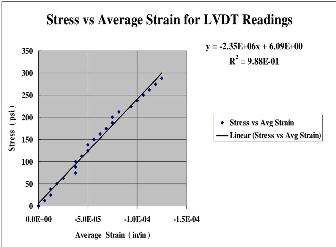
Figure 6 Stress versus Strain for Dog Bone 1
