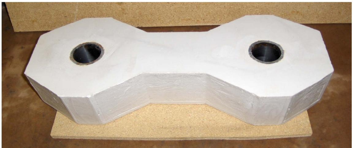
Figure 2 Hydro-Stone TB Specimen Dog Bone 1
