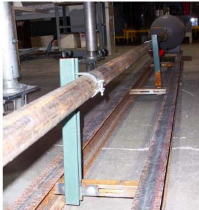
Figure 5.3 Air gun barrel and the I-Beam
