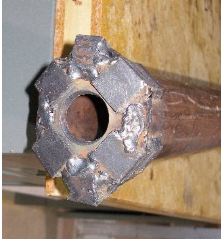
Figure 5.16 Final design of catch-tube with six L-clamps
