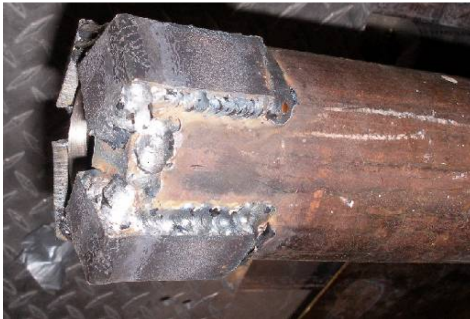
Figure 5.13 Deformed catch tube from the slug impact
