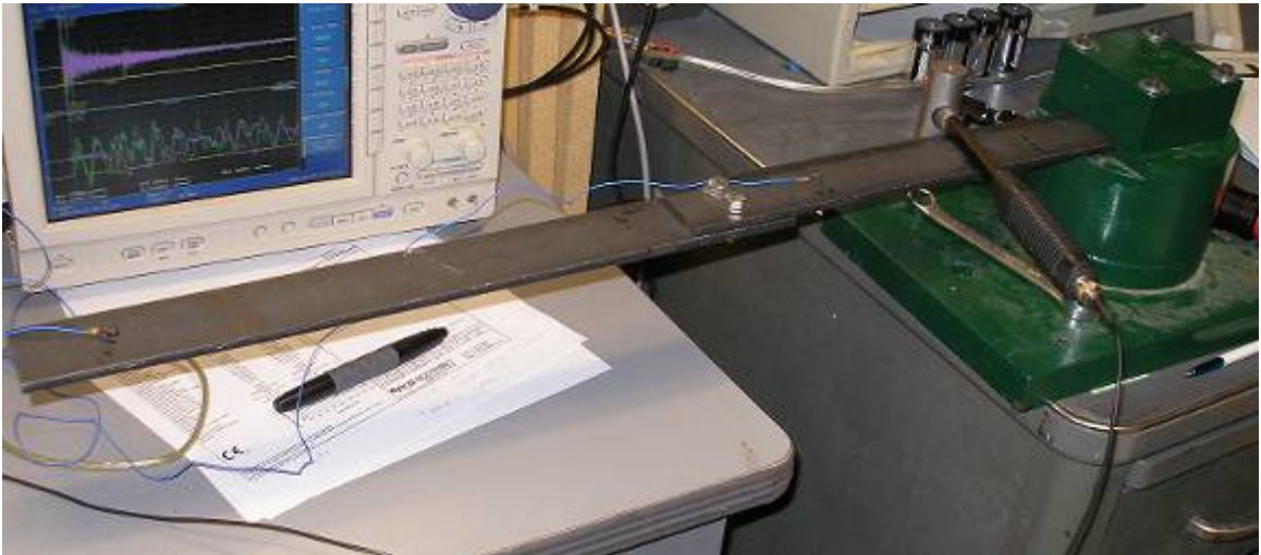
Figure 2.2 Cantilever beam with lap joint, support and accelerometers
