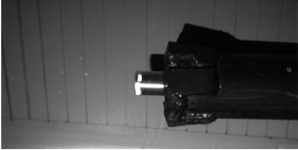
Figure 5.12 High speed camera image of slug and catch tube
