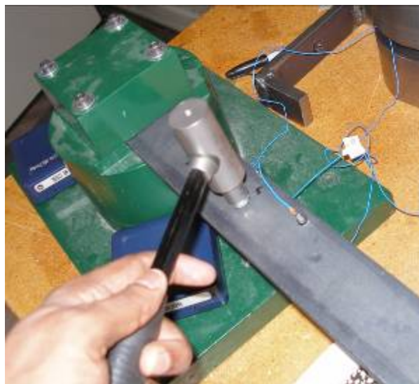
Figure 2.6 Impact hammer striking the cantilever beam
