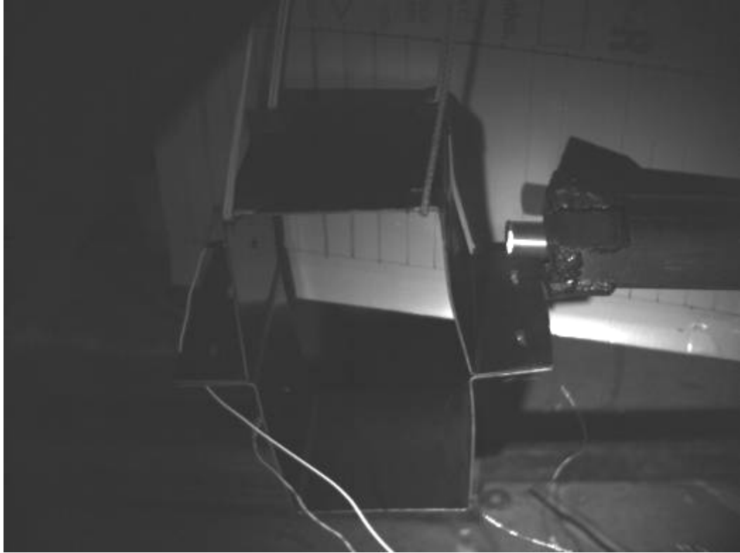
Figure 5.44 High speed camera image showing slug impacting the structure (4.33 ms after impact)
