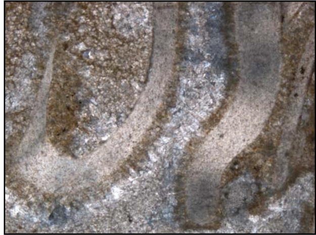
Figure 25: Needle-like acicular and equant cements, which grow at grain rims to fill pore spaces (seen here at the rims of bioclasts), are typical of phreatic-zone environments with some degree of freshwater input (Amieux et al., 1989).
