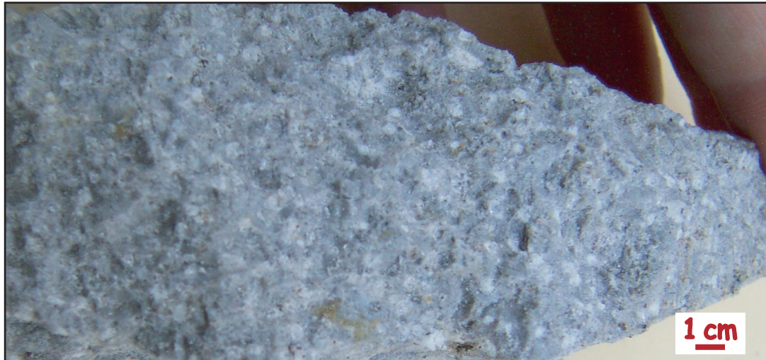
Figure 5.2. Pumiceous sample from the Gibbon River flow (GRWY7P). Sanidine, quartz, and plagioclase phenocrysts are visible.
