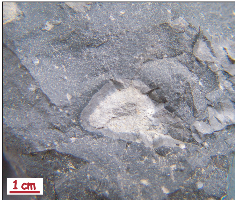
Figure 5.8. Basaltic enclave (light grey) with quenched rim (medium grey) in the mingled lava sample CSWY1 from the Crystal Spring flow.
