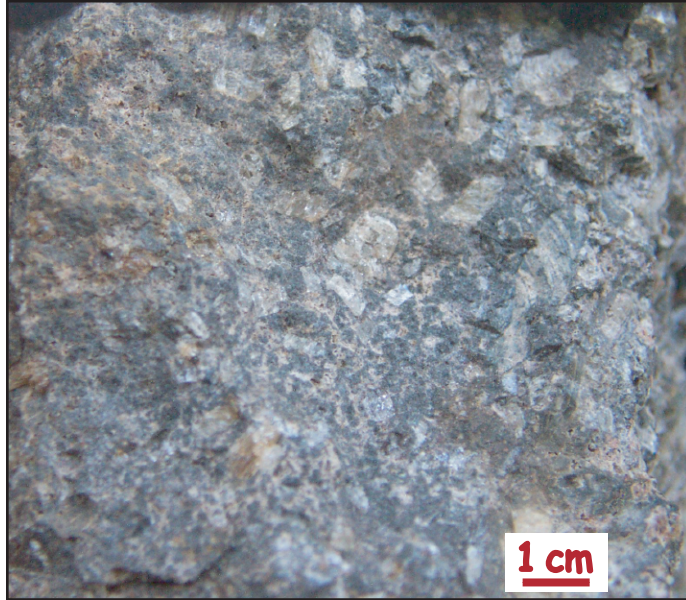
Figure 5.3. Porphyritic rhyolite sample from the Gibbon River flow (GRWY6). Sanidine and quartz phenocrysts are visible.
