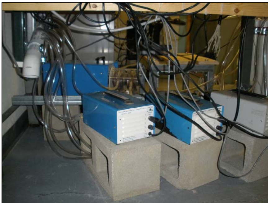
Figure 3.10 Pumps and plumbing of the evacuation system used to empty collection vessels
