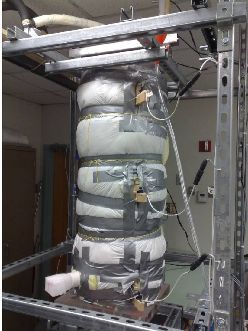
Figure 3.7 Test column covered with the insulation blanket. A high-density foam plug (left side bottom) is used to seal the port for circulating warm air to dry the column.
