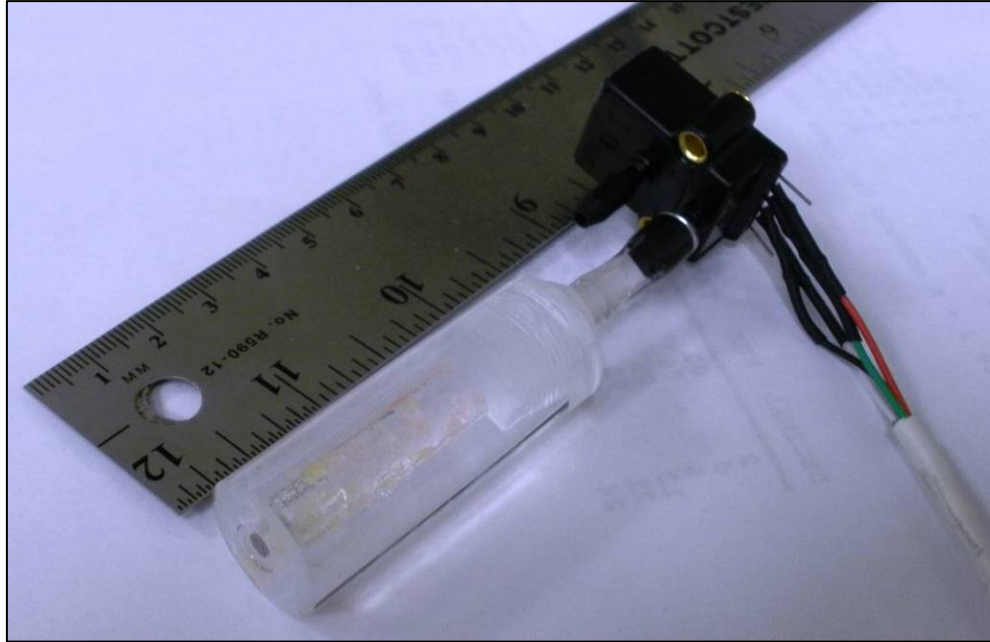
Figure 3.12 A tensiometer used to measure atmospheric tension inside the column. A porous metal plate is cemented to one end of the water-filled hole in the acrylic rod. The other end of the hole is connected to a 15 psi pressure transducer.
