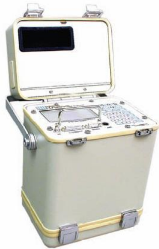
Figure 3-6 Photograph of the portable TRASE unit for measuring soil moisture.
