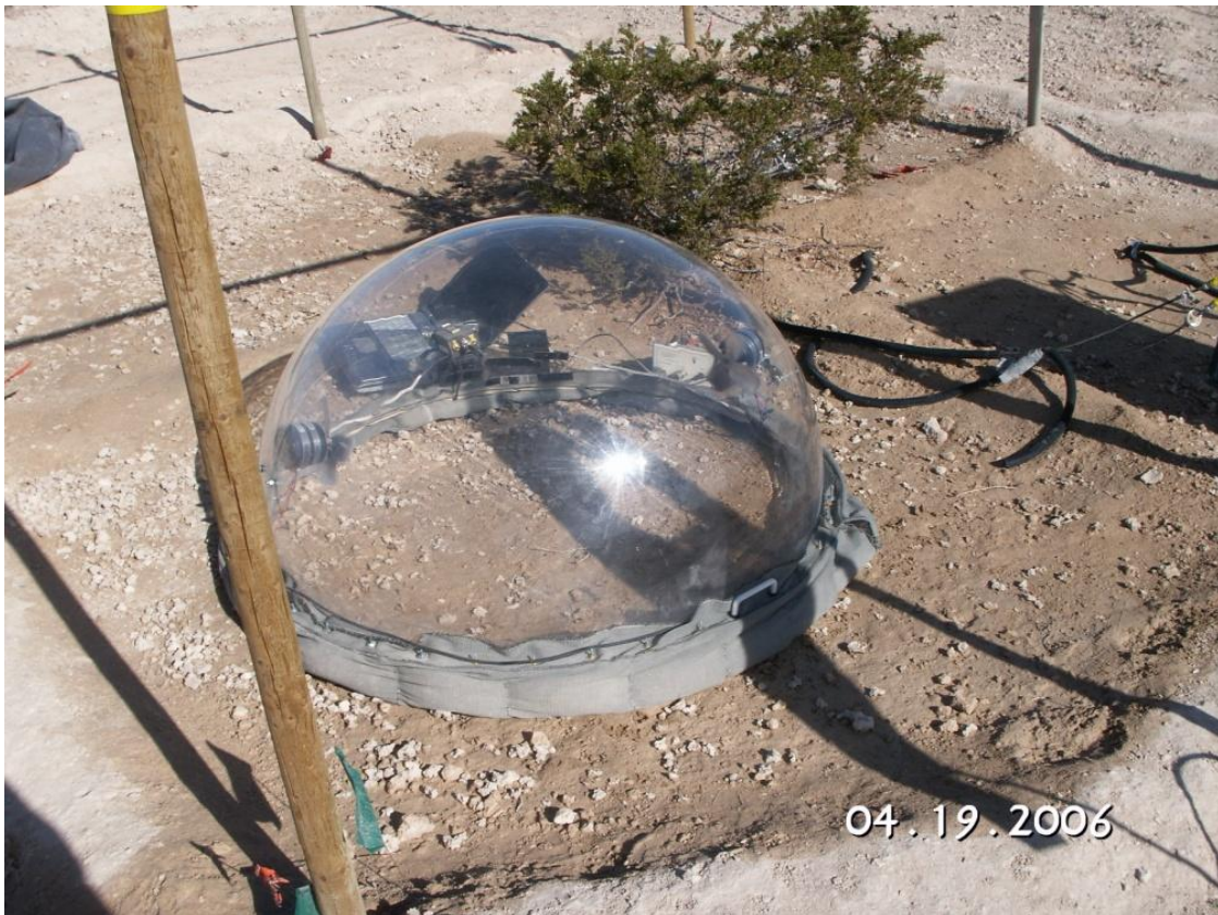
Figure 3-10 Portable vapor pressure dome used for measuring soil water evaporation fluxes.
