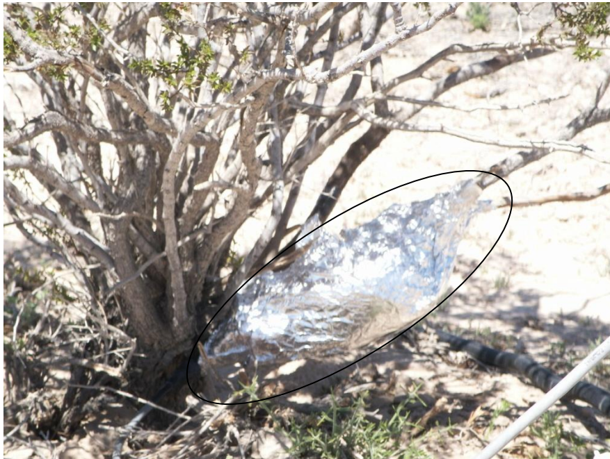
Figure 3-13 Stem flow gage and leading stem wrapped in thermal resistant and solar reflective materials (circled) attached to a creosote bush stem.
