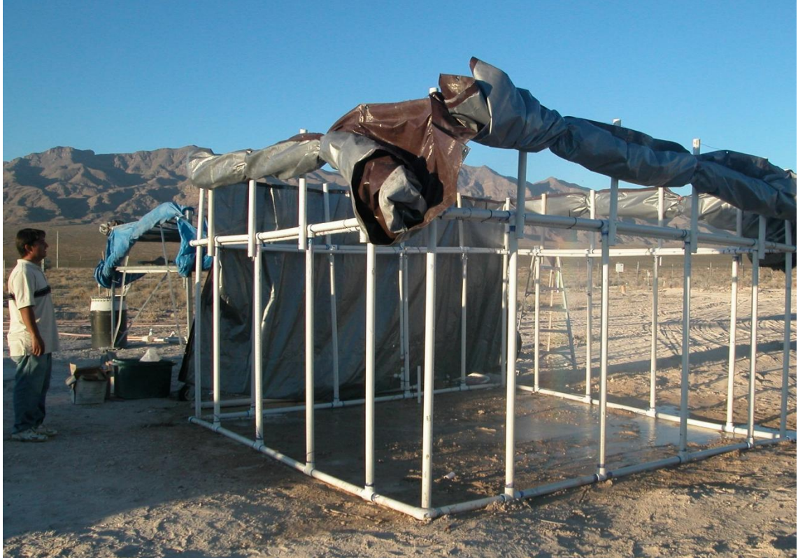
Figure 3-3 Photograph of a newly constructed rainfall simulator during preliminary testing of precipitation rates.
