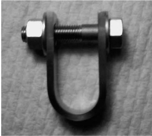
Figure 2.8 Pictorial View of U-bend Specimen
