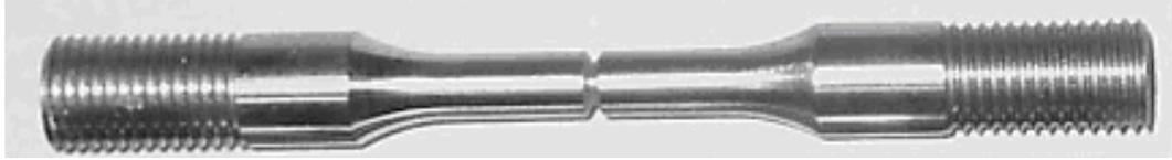
Figure 2.3 Pictorial View of Notched Cylindrical Specimen
