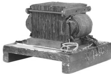
Figure 2.2 William Stanley's Original Transformer, circa 1885 [7]
