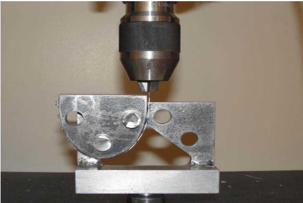
Figure 3.10 Picture of Archwire Engaged in Ceramic Bracket Arc-Form Set Up
