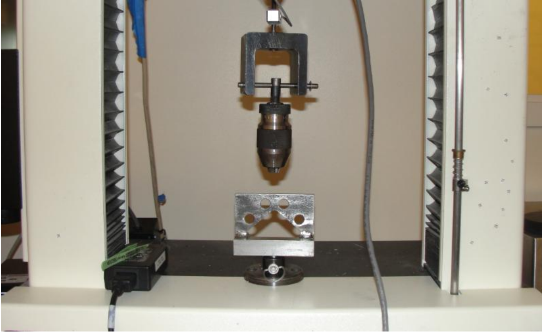
Figure 3.9 Picture of Universal Testing Machine with Set-up
