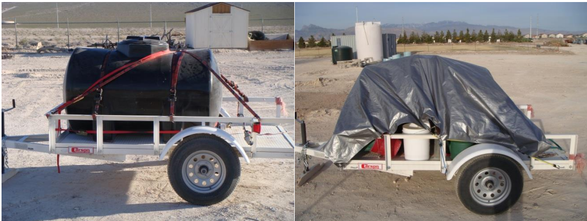
Figure 4. Tank for storage of post-UV reclaimed water.
