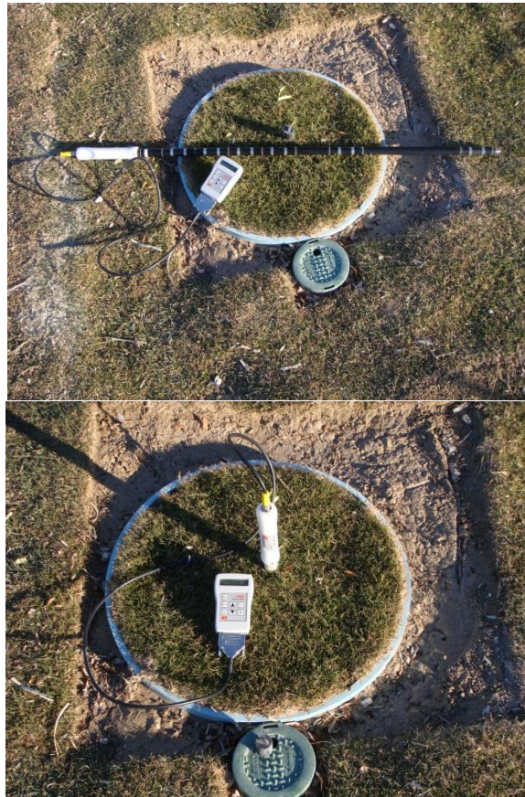
Figure 3. Profiler access probe to show length and installation into access tube.
