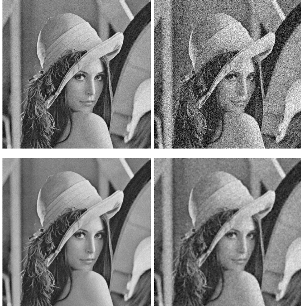
Fig.5.7 First row: “Lena” image with noise level \sigma = 10 and 40; Second row: Corresponding SWCD results
