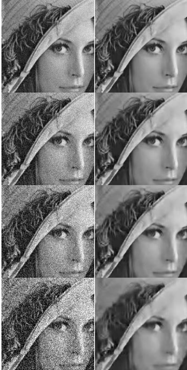
Fig. 6.7 First column: “Lena” image with AWG noise, \sigma=10, 20, 30, and 50 ; Second column: corresponding results by the LFAD.
