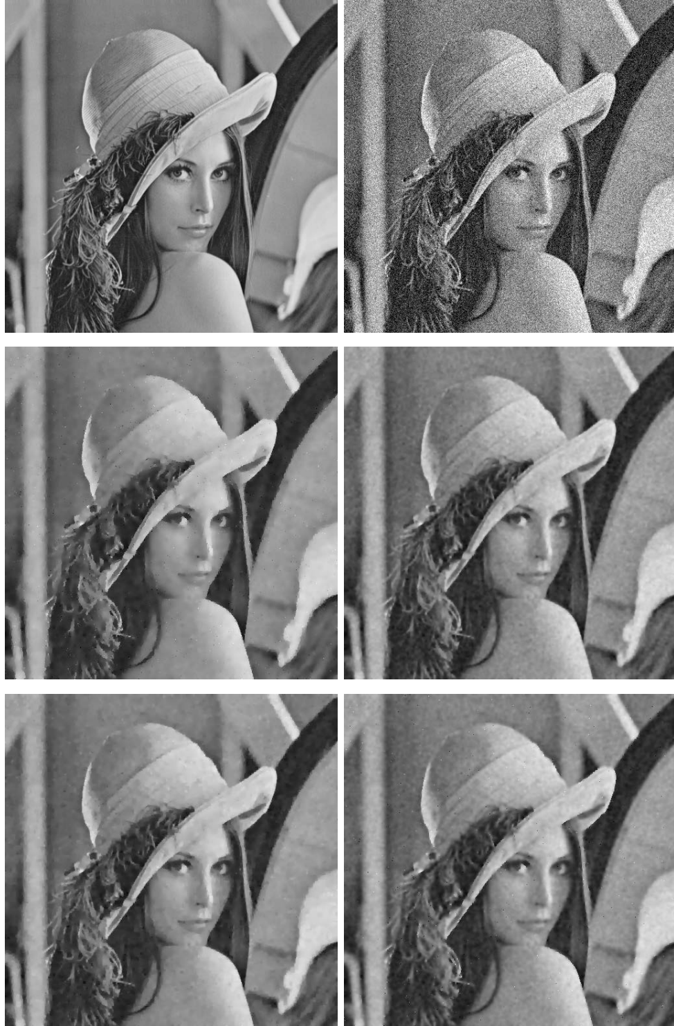
Fig. 3.2 First row: “Lena” image and that with AWG noise, \sigma = 30 ; Second row: Results by Cauchy and Fair; Third row: Results by L1-L2 and Welsch.
