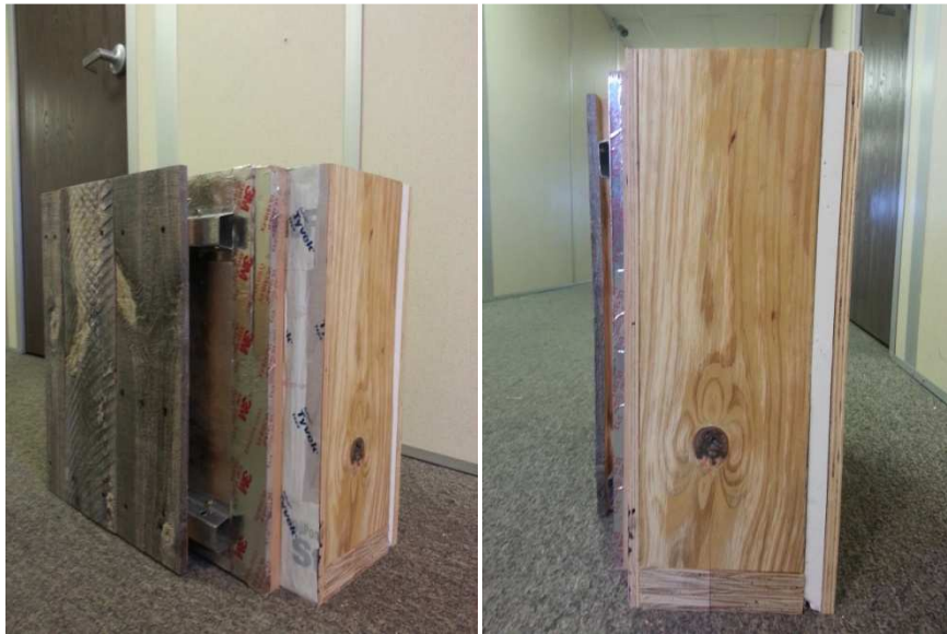
Figure 4. Exterior Wall Sections
