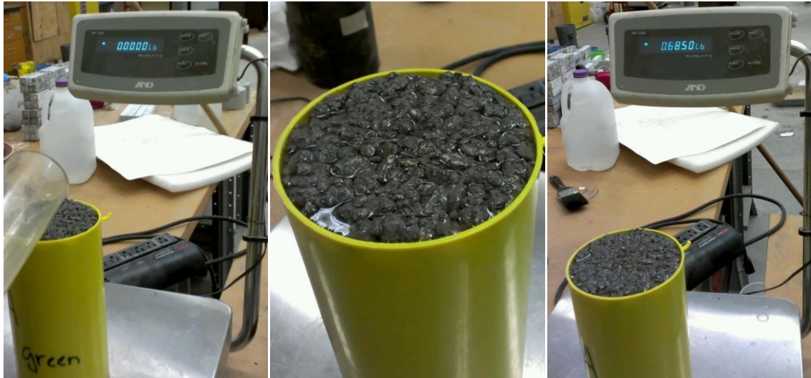
Figure 3.8. Images of porosity testing process
