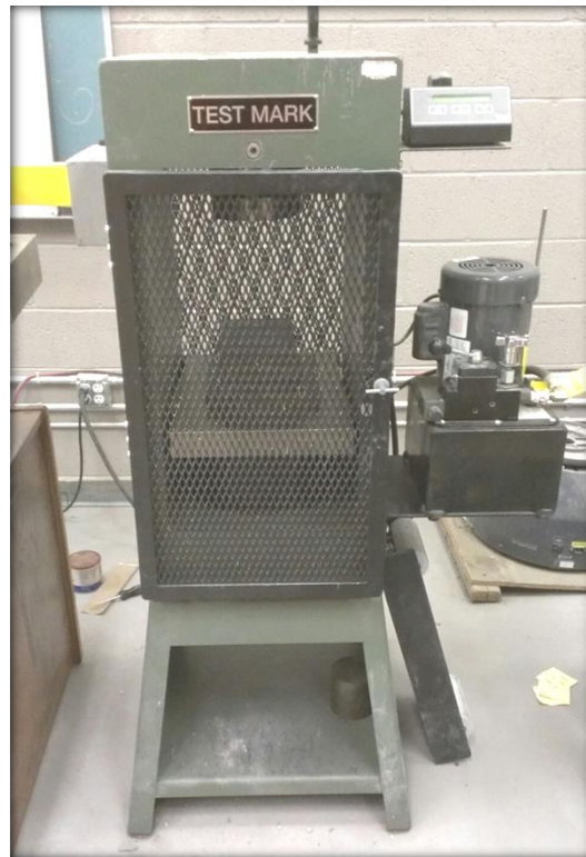
Figure 3.6. Loading machine used for compression and tensile tests
