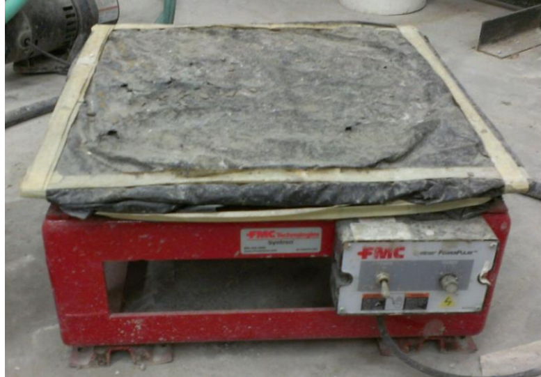
Figure 3.3. Machine used to assist in concrete compaction
