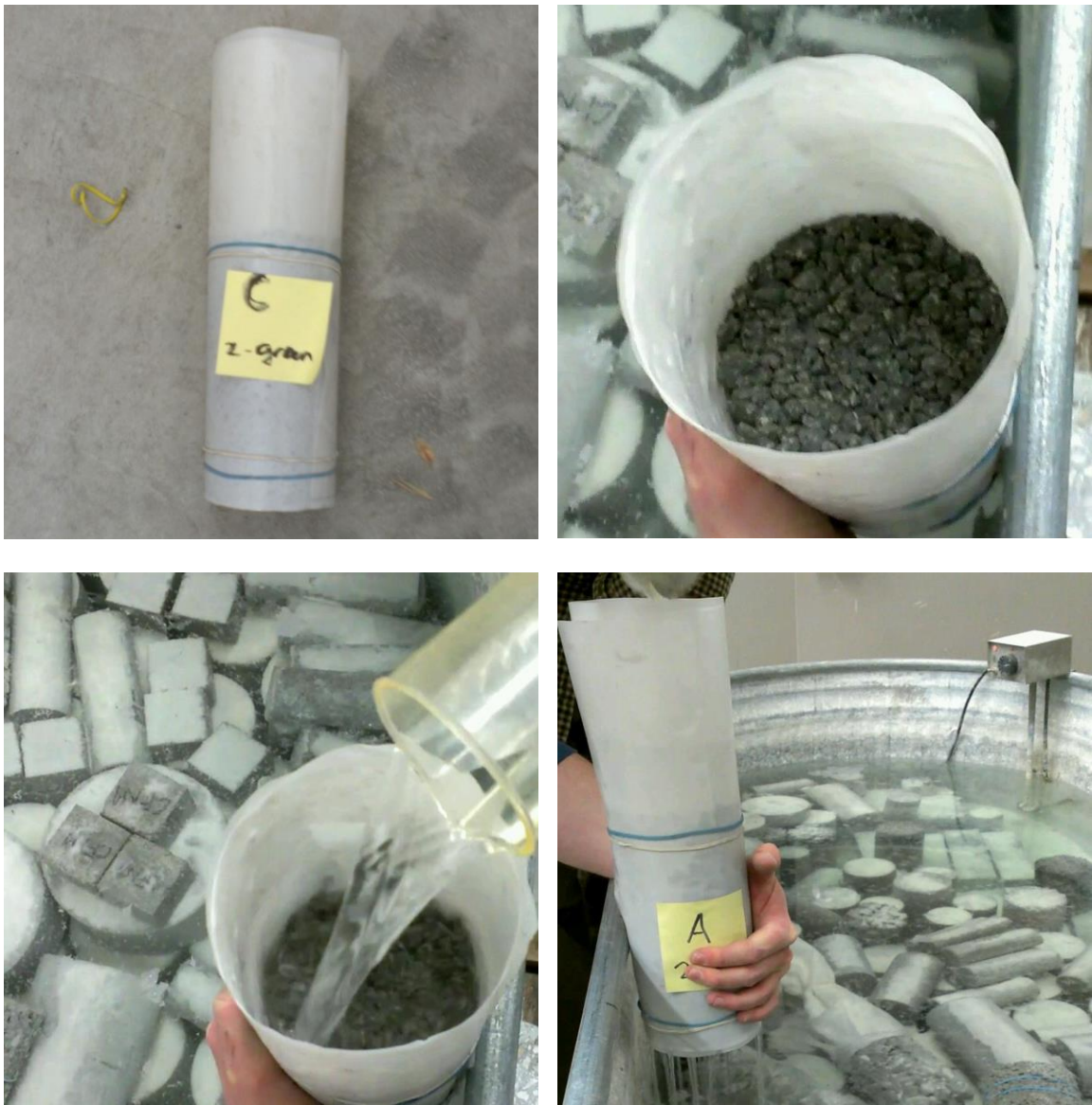
Figure 3.9. Various stages of the permeability testing process
