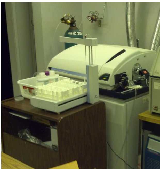
Figure 11. ELAN DRC II ICP-MS coupled with S-10 Autosampler
