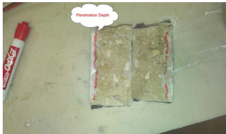
Figure 3.15: Chloride Penetration Depth after Applying Silver Nitrate to the Freshly Split Sections
