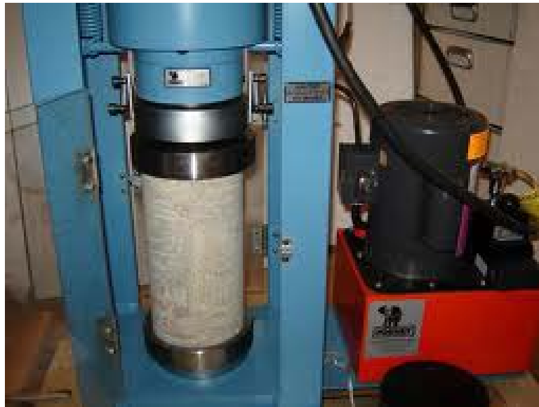
Figure 3.7: Concrete Cylinder Experiencing Axial Load
