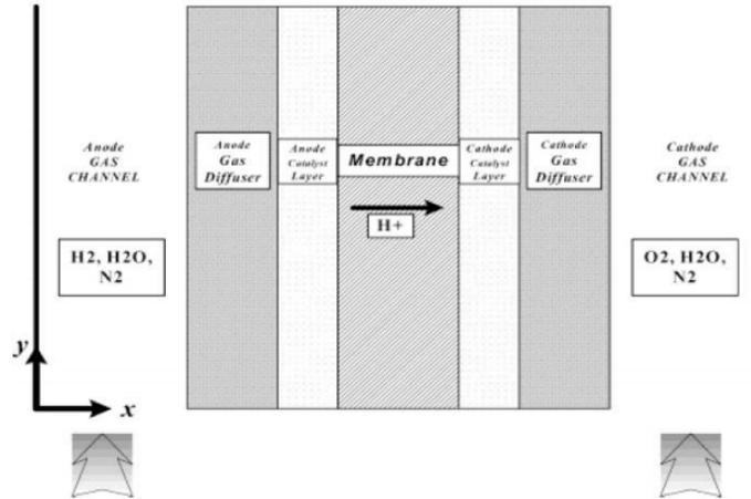
Figure 3.1. A schematic 2D PEMFC [Wang (2004)]
