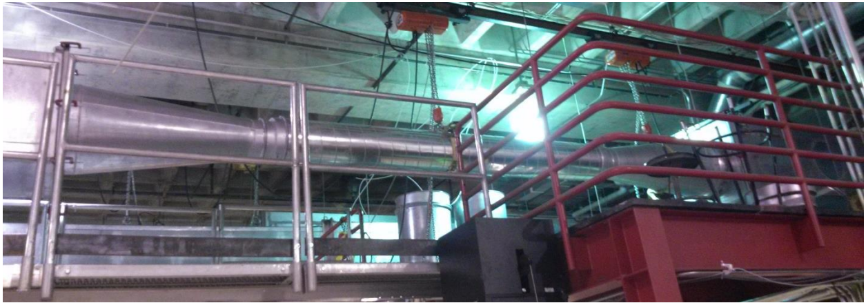
Figure 5.4: 12-in Diameter Duct Test Setup
