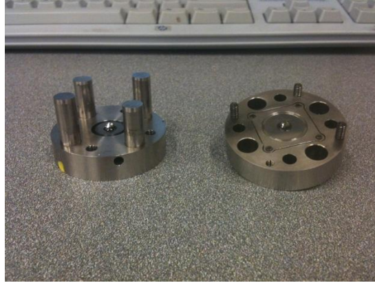
Figure 34. A four-posts wide-opening DAC. Designed for single crystal measurements.
