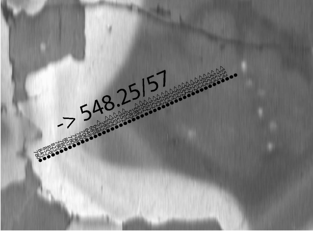
Figure A37 EPMA capture of site 9 on Sample 136-2B. Each black dot is a point analyzed for Ti concentration followed by the TitaniQ result at a\text{TiO}_2 = 0.6 . The length of the traverse is 548.25 \mu\text{m} and has 57 points. The arrow indicates the opposite direction of the traverse. Table A82 has the corresponding EPMA and TitaniQ data.
