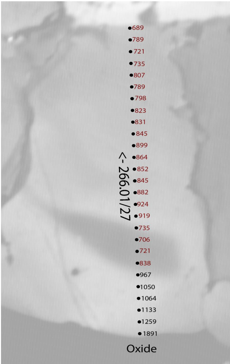
Figure A22 EPMA capture of site 5A on Sample 136-1A. Each black dot is a point analyzed for Ti concentration followed by the TitaniQ result at a\text{TiO}_2 = 0.6 . Red numbers represent good data, while black numbers represent targets that are too close to an oxide for accurate analysis. The length of the traverse is 266.01\mu\text{m} and has 27 points. The arrow indicates the direction of the traverse. Table A68 has the corresponding EPMA and TitaniQ data.
