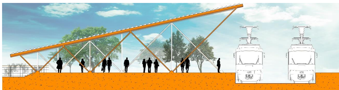
Fig. 5.2, Schematic section illustrating the roof structure upon which the AWG could be integrated as a means of water collection. A particularly large roof area translates to more PV power that can operate additional AWG units, leading to more water collected.
