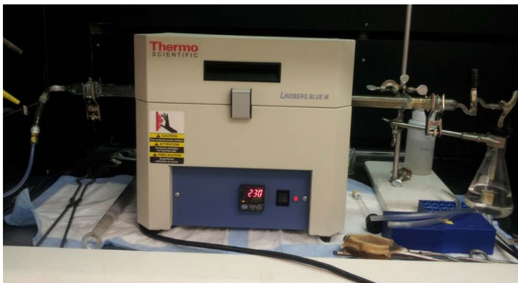
Figure 5. Tube furnace set-up inside fume hood for U 3 O 8 synthesis
