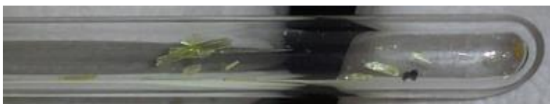
Figure 4.1 \text{Tc}_2\text{O}_7 crystals in sealed tube obtained after the oxidation of \text{TcO}_2 by \text{O}_2 at 450^\circ\text{C} .
