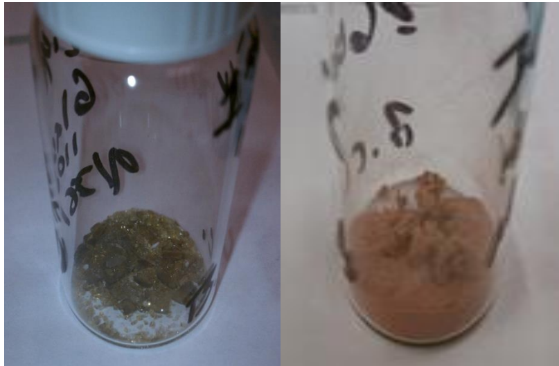
Figure 3.3. Glass prepared under flowing air at 800 ° (right) and at 1100 °C (left).
