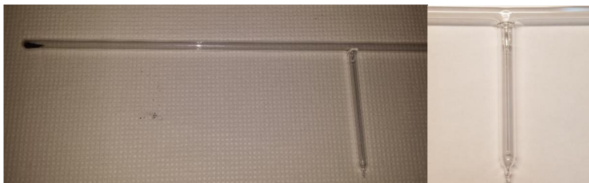
Figure 2.8. Specialty reaction tube with TcO_2 (right) and the small capillary inside of Pyrex casing (left). The capillary was made from standard 2 mm outer diameter (OD) Pyrex tubing. The closed (test tube) end was submerged in 48% aqueous HF until the OD was reduced to 1.96 mm. This exactly matches the OD of the aluminum sample cups that fit into the MS probe.
