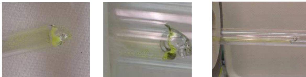
Figure 1.18. From left to right are images of solid, liquid, and gaseous \text{Tc}_2\text{O}_7 .
