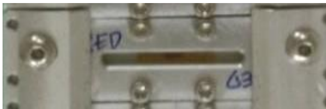
Figure 2.9. XAFS sample holder for solid-state compound.
