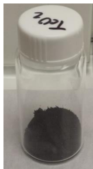
Figure 2.2. Technetium dioxide stored in a scintillation vial.
