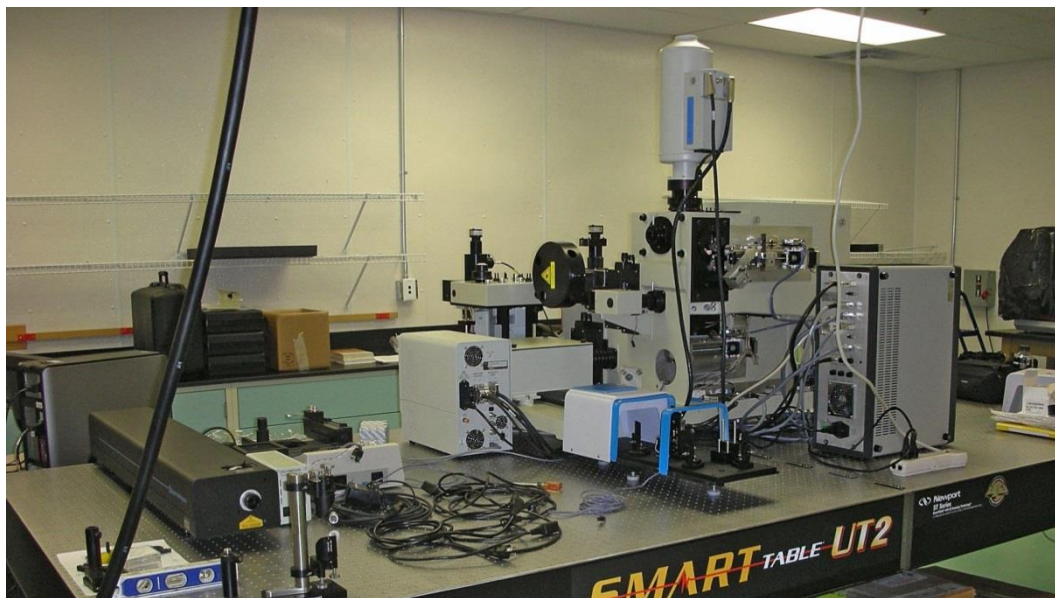
Figure 2.13. Jobin-Yvon Horiba T-64000 Raman Spectrometer (UNLV).
