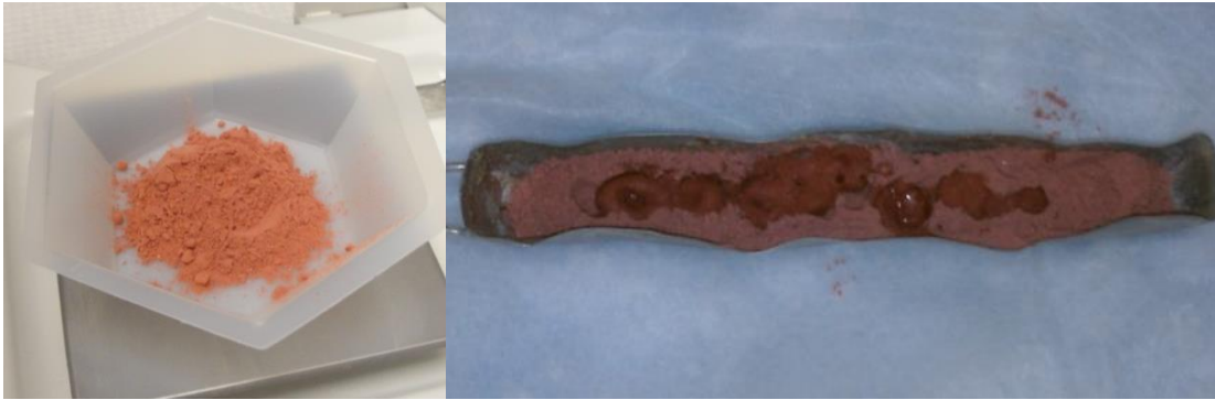
Figure 3.2. Glass batch before (left) and after (right) adding the technetium solution.
