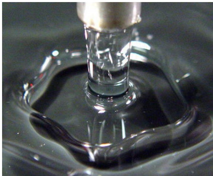
Figure 4 - Hydraulic Jump Forming Around a Faucet (Bush & Aristoff, 2008)
