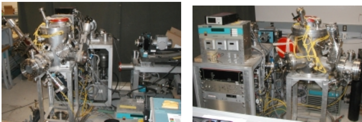
Figure 8. Existing vacuum system in the Electromagnetics Laboratory. Vacuum system includes a turbomolecular pump, roughing pump, a cryogenic pump, controls and gauges, and a VUV grazing incidence monochromator/spectrograph
