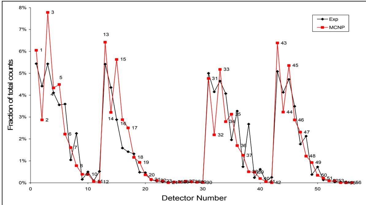
**Figure 3. AT-1, Fraction of Total Counts by Detector Number, MCNPX vs. Experiment.** Side detectors are 13-24 and 31-42, top detectors are 1-12, bottom detectors are 31-42.
