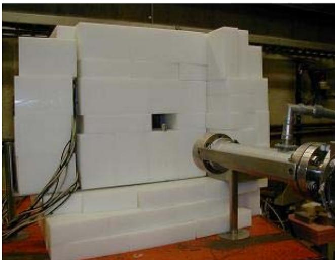
**Figure 1. Front of Bcube.** The AmBe source can be seen in the opening. The beam height had not been adjusted in this photograph.
