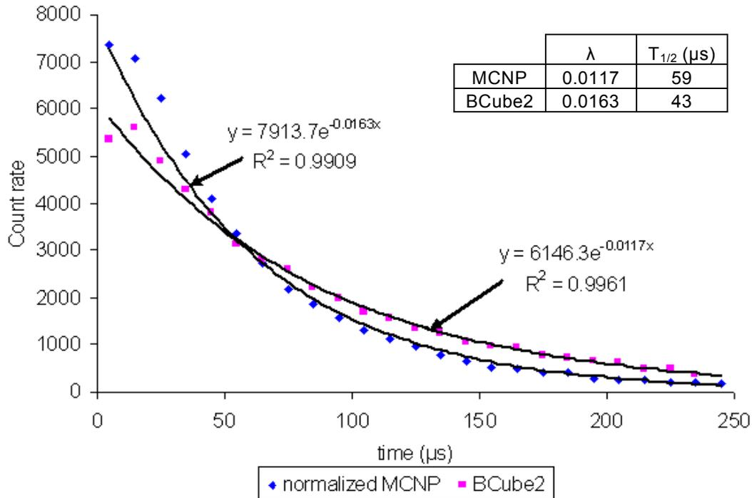
**Figure 2. BCube2 Lifetime.** A numerical fit of neutron capture times for BCube2. Calculated lifetimes from experimental data and from MCNPX are also shown.
