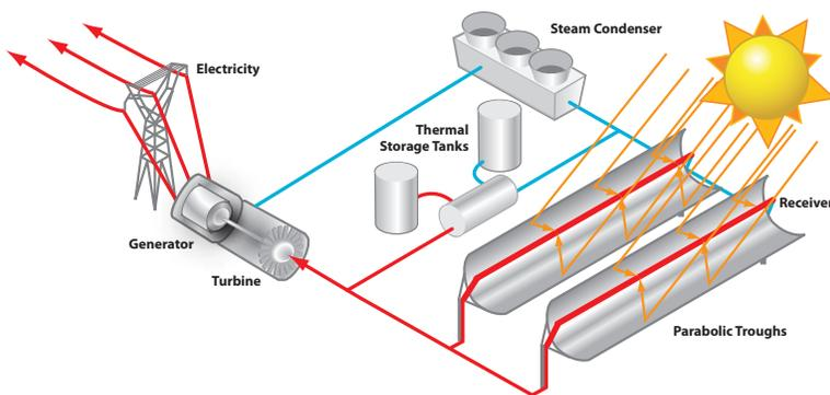
Simplified schematic of a parabolic trough CSP plant with thermal energy storage tanks. Excess solar energy is stored as hot fluid in the tanks during the day and released to power the turbine and make electricity during cloudy periods or at night.
