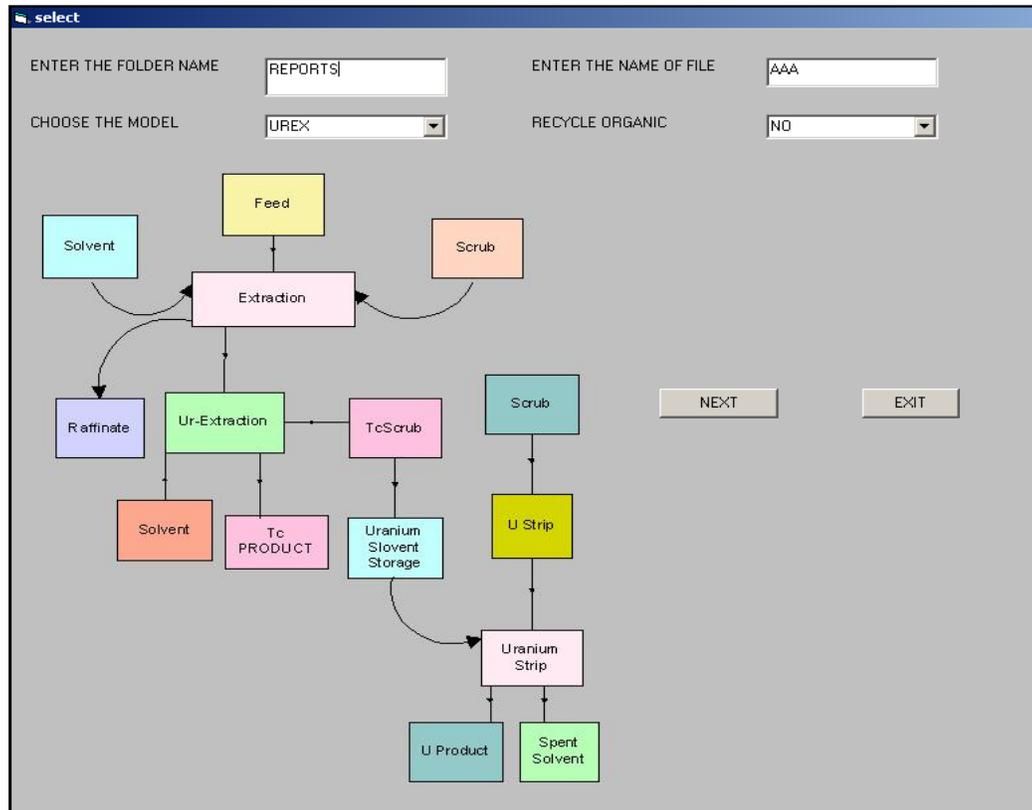
**Figure 2 - GUI for user selection of predefined processes.**
