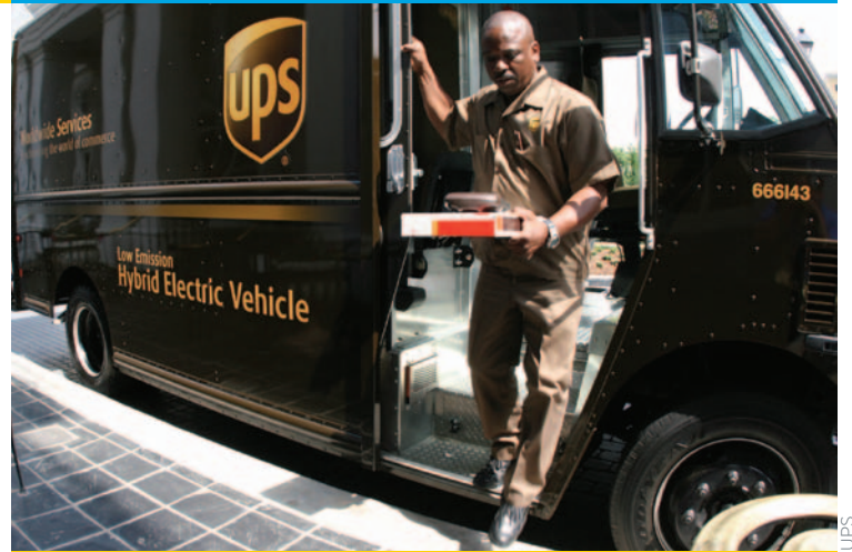
UPS' hybrid electric delivery vans demonstrate 31% to 37% higher fuel economy than comparable conventional vans.
