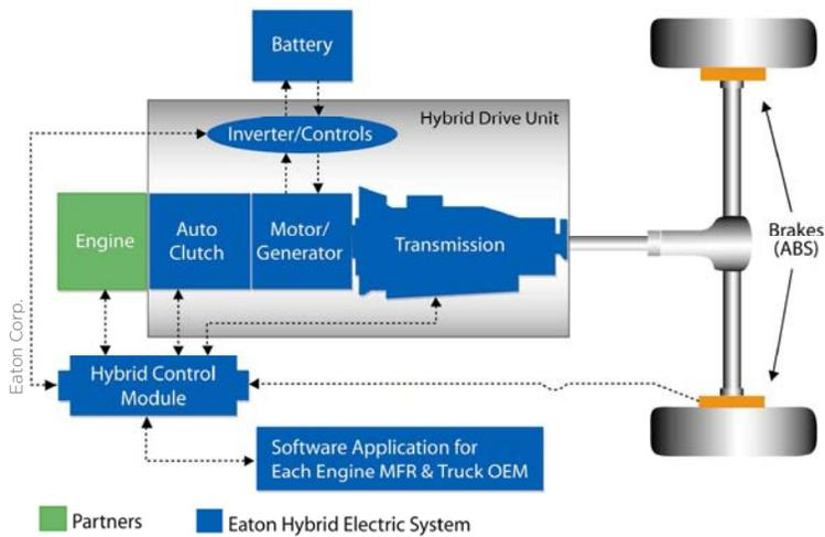
Eaton Corp.'s parallel hybrid system is found in UPS hybrid electric delivery vans.
