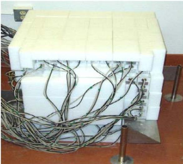
Figure 1. NMDS in the cubic configuration for cosmic radiation measurements.
