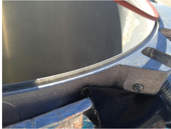
Figure 16: Machined groove for O-ring
