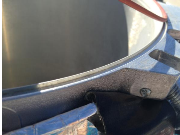
Figure 16: Machined groove for O-ring
