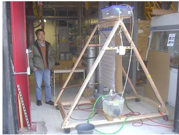
Figure 10. Photobioreactor of hanging bag
