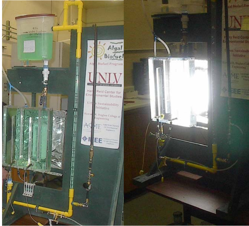
Figure 11. small scale flat Photobioreactor.
