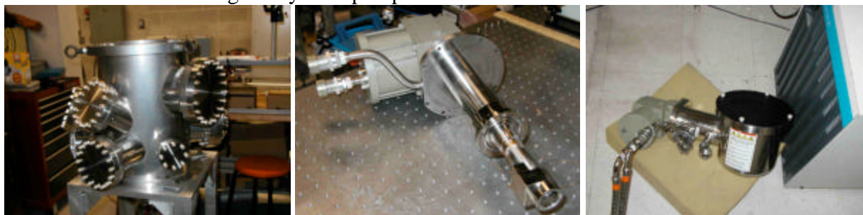
Figure 3. Vacuum Chamber, Cryogenic Pump, and Cryostat to be used for SEE Tests.
