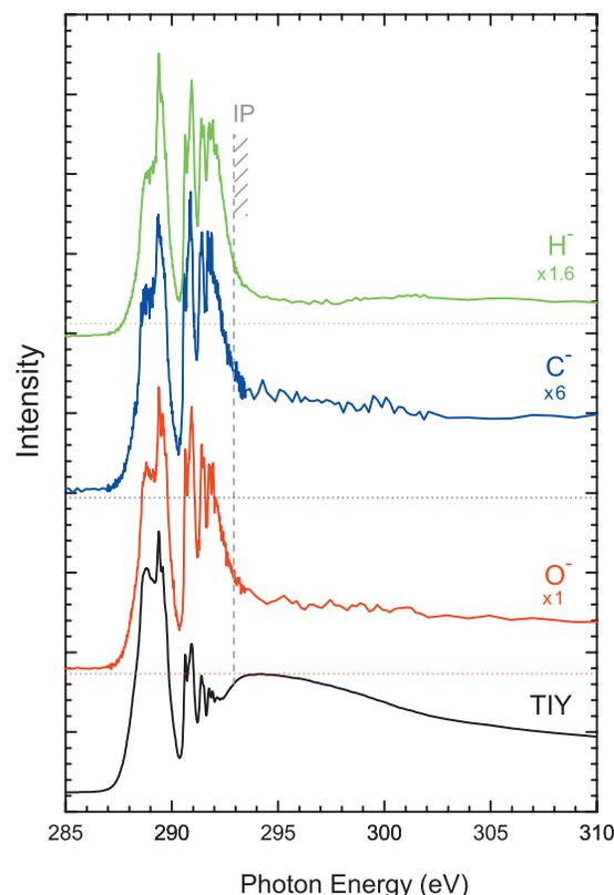
FIG. 6. Partial yields for  $\text{H}^-$ ,  $\text{C}^-$ , and  $\text{O}^-$  negative ion fragments (anions) following photoexcitation of  $\text{C}_2\text{H}_4\text{O}$  near the C  $1s$  ionization threshold, the TIY is added for comparison. Numerical values are approximate intensity values relative to the O-anion fragment at 295 eV.
