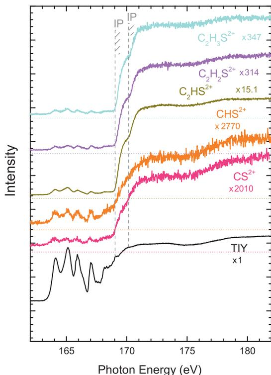
FIG. 12. Partial yields for  $C_2H_3S^{2+}$ ,  $C_2H_2S^{2+}$ ,  $C_2HS^{2+}$ ,  $CHS^{2+}$ , and  $CS^{2+}$  ion fragments (cations) following photoexcitation of  $C_2H_4S$  near the  $S\ 2p$  ionization thresholds, the TIY is added for comparison. Numerical values are approximate intensity values relative to the TIY at 173 eV.
