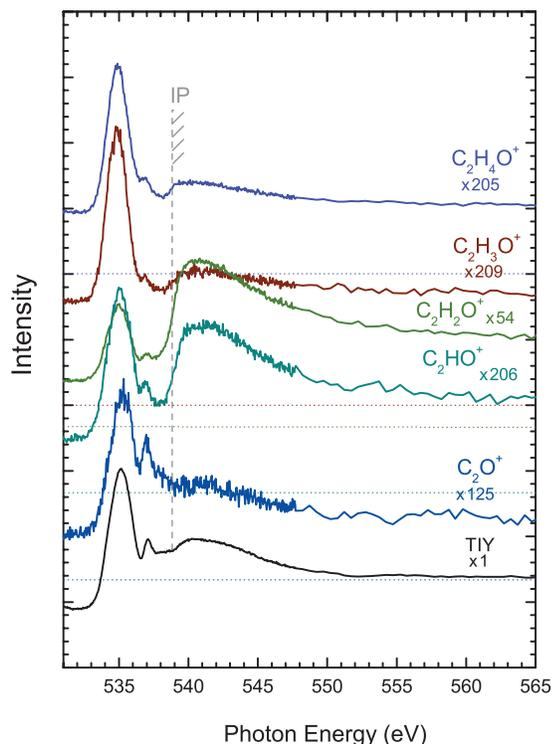
FIG. 7. Partial yields for  $C_2H_4O^+$ ,  $C_2H_3O^+$ ,  $C_2H_2O^+$ ,  $C_2HO^+$ , and  $C_2O^+$  ion fragments (cations) following photoexcitation of  $C_2H_4O$  near the  $O\ 1s$  ionization threshold, the TIY is added for comparison. Numerical values are approximate intensity values relative to the TIY at 555 eV.
