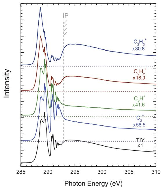
FIG. 3. Partial yields for  $C_2H_3^+$ ,  $C_2H_2^+$ ,  $C_2H^+$ , and  $C_2^+$  ion fragments (cations) following photoexcitation of  $C_2H_4O$  near the C  $1s$  ionization threshold, the TIY is added for comparison. Numerical values are approximate intensity values relative to the TIY at 295 eV.
