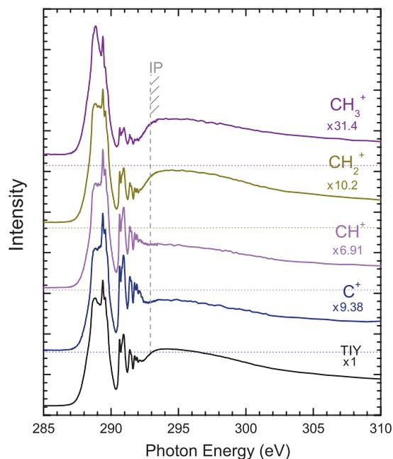
FIG. 4. Partial yields for  $CH_3^+$ ,  $CH_2^+$ ,  $CH^+$ , and  $C^+$  ion fragments (cations) following photoexcitation of  $C_2H_4O$  near the C  $1s$  ionization threshold. Numerical values are approximate intensity values relative to the TIY at 295 eV.
