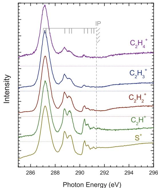
FIG. 9. Partial yields for  $C_2H_4^+$ ,  $C_2H_3^+$ ,  $C_2H_2^+$ ,  $C_2H^+$ , and  $S^+$  ion fragments (cations) following photoexcitation of  $C_2H_4S$  near the C  $1s$  ionization threshold. The spectra are normalized on the transition near 287.2 eV.
