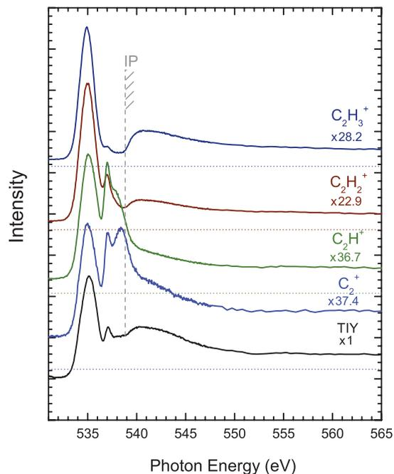
FIG. 8. Partial yields for  $C_2H_3^+$ ,  $C_2H_2^+$ ,  $C_2H^+$ , and  $C_2^+$  ion fragments (cations) following photoexcitation of  $C_2H_4O$  near the  $O\ 1s$  ionization threshold, the TIY is added for comparison. Numerical values are approximate intensity values relative to the TIY at 555 eV.
