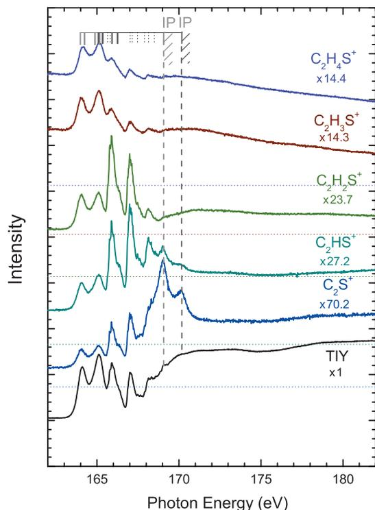
FIG. 10. Partial yields for  $C_2H_4S^+$ ,  $C_2H_3S^+$ ,  $C_2H_2S^+$ ,  $C_2HS^+$ , and  $C_2S^+$  ion fragments (cations) following photoexcitation of  $C_2H_4S$  near the S  $2p$  ionization thresholds, the TIY is added for comparison. Numerical values are approximate intensity values relative to the TIY at 173 eV.
