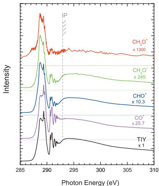
FIG. 2. Partial yields for  $CH_3O^+$ ,  $CH_2O^+$ ,  $CHO^+$ , and  $CO^+$  ion fragments (cations) following photoexcitation of  $C_2H_4O$  near the C  $1s$  ionization threshold, the TIY is added for comparison. Numerical values are approximate intensity values relative to the TIY at 295 eV.
