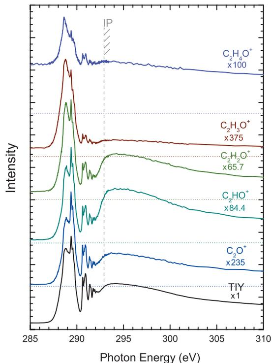
FIG. 1. Partial yields for  $C_2H_4O^+$ ,  $C_2H_3O^+$ ,  $C_2H_2O^+$ ,  $C_2HO^+$ , and  $C_2O^+$  ion fragments (cations) following photoexcitation of  $C_2H_4O$  near the C  $1s$  ionization threshold, the TIY is added for comparison. Numerical values are approximate intensity values relative to the TIY at 295 eV.
