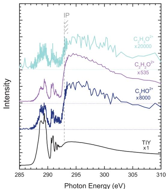
FIG. 5. Partial yields for  $\text{C}_2\text{H}_3\text{O}^{2+}$ ,  $\text{C}_2\text{H}_2\text{O}^{2+}$ , and  $\text{C}_2\text{HO}^{2+}$  ion fragments (cations) following photoexcitation of  $\text{C}_2\text{H}_4\text{O}$  near the C  $1s$  ionization threshold, the TIY is added for comparison. Numerical values are approximate intensity values relative to the TIY at 295 eV.
