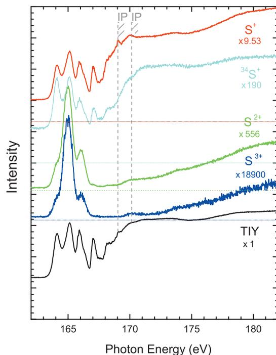
FIG. 13. Partial yields for  $S^+$ ,  $S^{2+}$ , and  $S^{3+}$  ion fragments (cations) following photoexcitation of  $C_2H_4S$  near the  $S\ 2p$  ionization thresholds, the TIY is added for comparison. Numerical values are approximate intensity values relative to the TIY at 173 eV.
