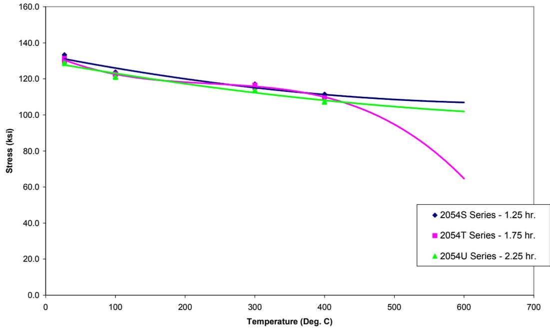
Figure 1.3.3. Ultimate Tensile Strength versus Test Temperature
