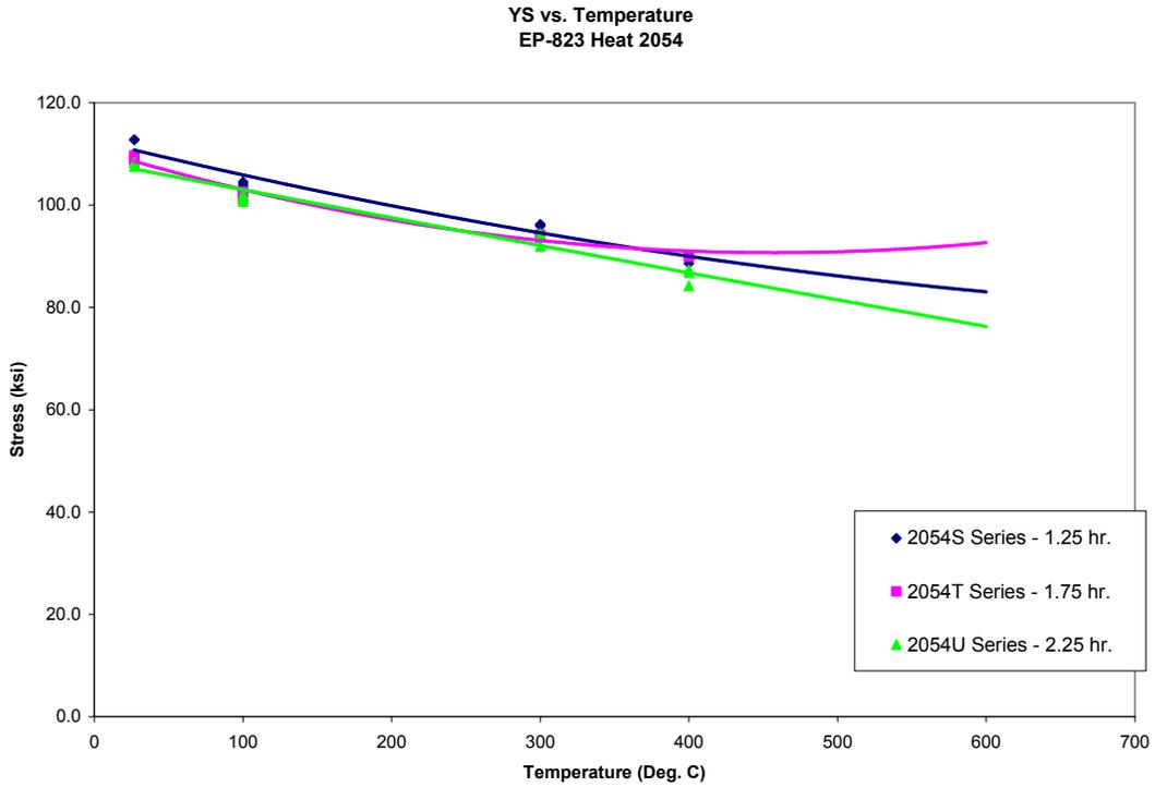
Figure 1.3.2. Yield Strength versus Test Temperature
